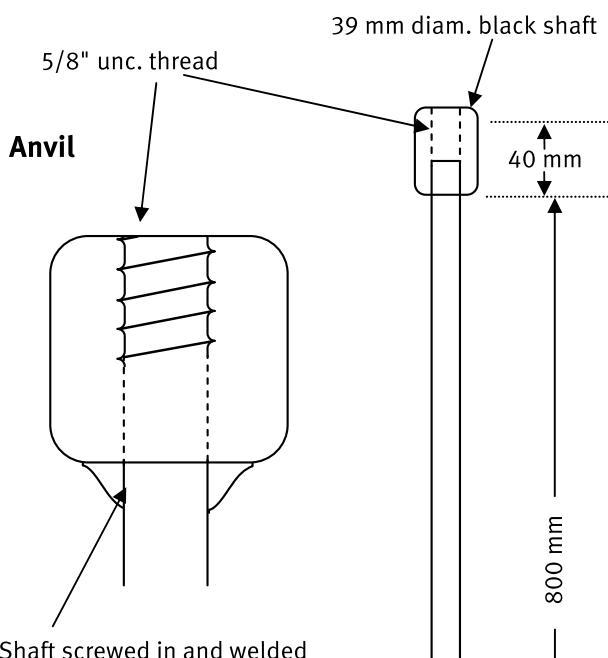
Shaft screwed in and welded
