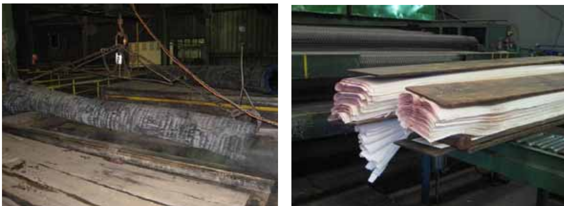
Figure 11. Processing of Khaya logs into sliced veneer.
