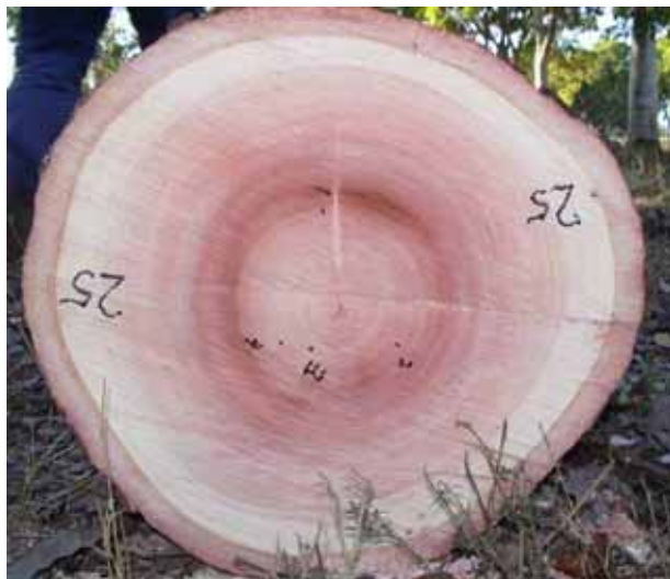
Figure 5. Transverse face of a Khaya log end soon after felling with distinctive heartwood, transition wood and sapwood zones (the small numbers - 1, 2, 3 and 4 - denote small end splits that were measured). Such distinctiveness was not observed in all log ends.
