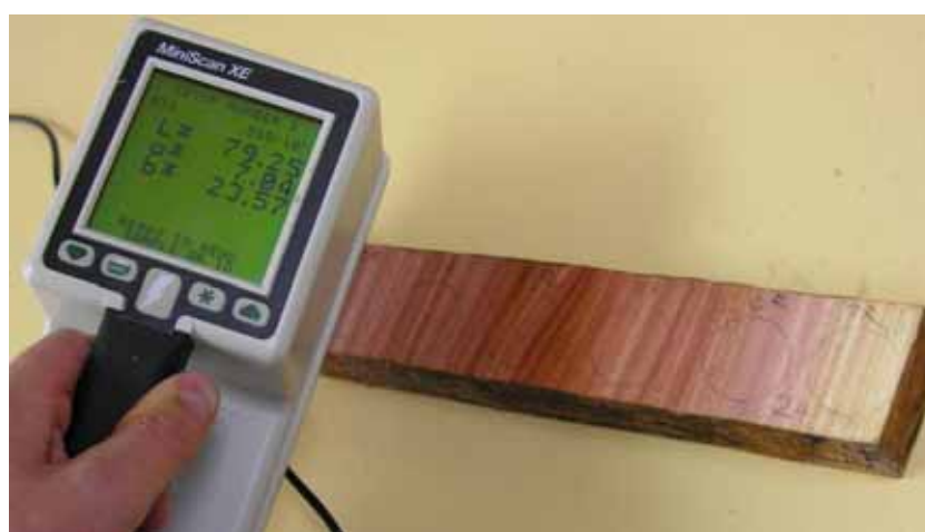
Figure 6. MiniScan XE portable spectrometer in use. Note the circular spots marked on the wood sample representing heartwood, transition wood and sapwood assessment points.
