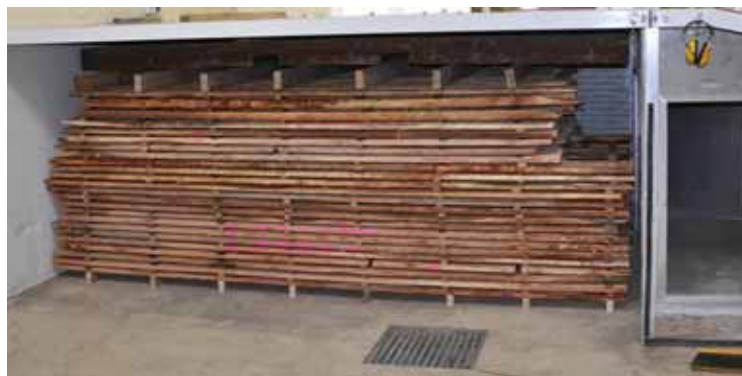
Figure 8. Timber loaded in kiln with concrete weight for restraint.
