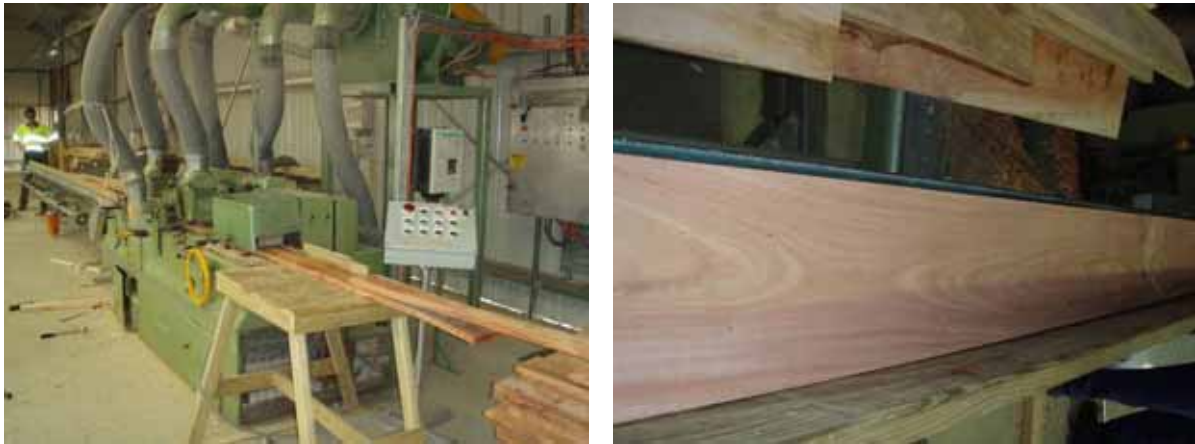
Figure 9. Moulding boards to final dimensions.
