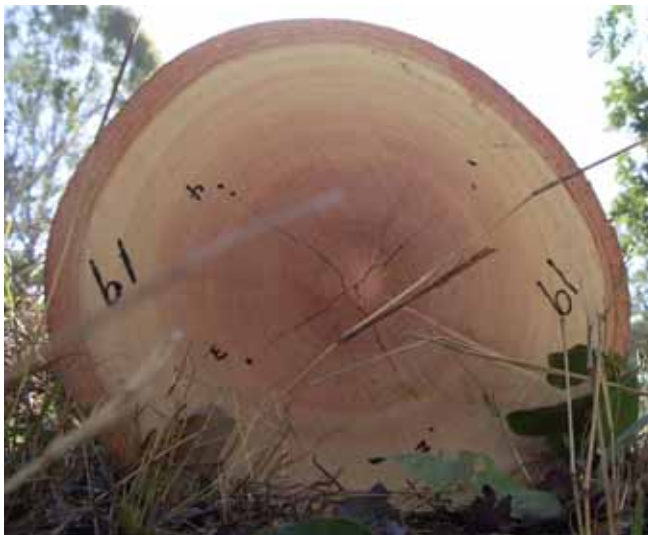
Figure 4. The large end of tree number 19 from the 18-year-old plot at Burdekin Agricultural College showing end-splitting and pen numbers and radial measure points marked at initial assessment and at the second assessment when the crack had propagated further.
