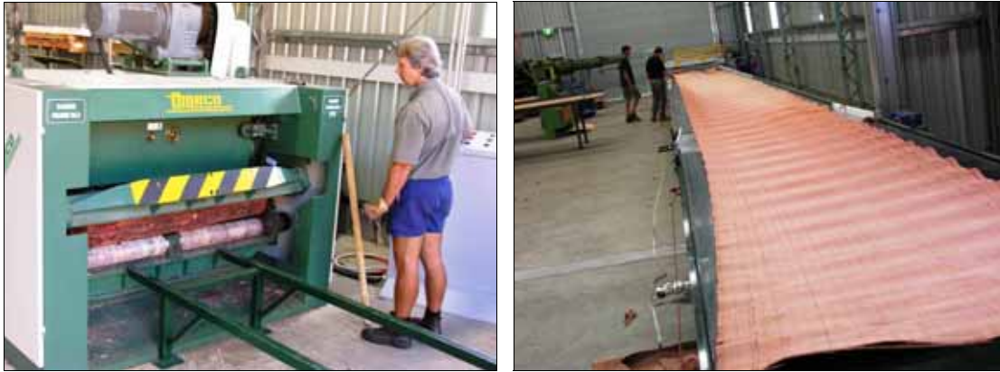
Figure 10. Processing of Khaya billets into veneer sheet using Omeco spindleless lathe.
