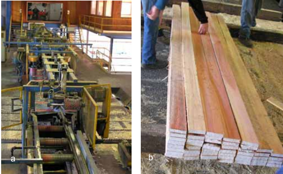
Figure 7. Vislander sawmill headrig (a); the final sawn product (b).
