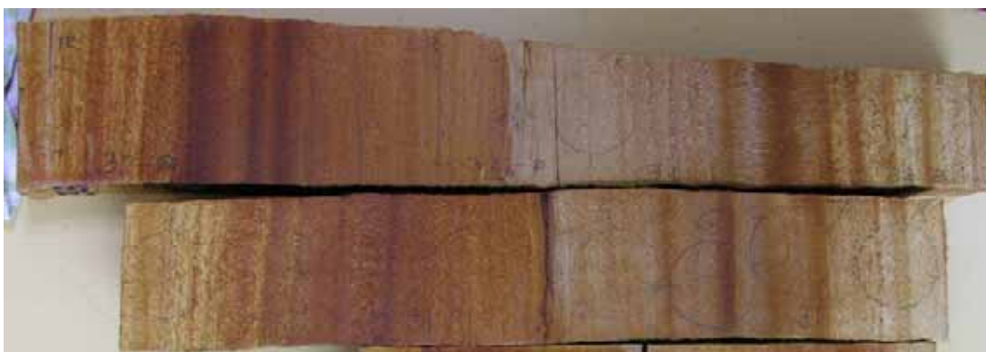
Figure 19. Two samples coated with different surface finish treatments - right-hand halves of both samples are untreated; lacquer finishing was applied to the left-hand side of the upper sample and Danish oil was applied to the left-hand side of the bottom sample. Further details are provided in the text above.
