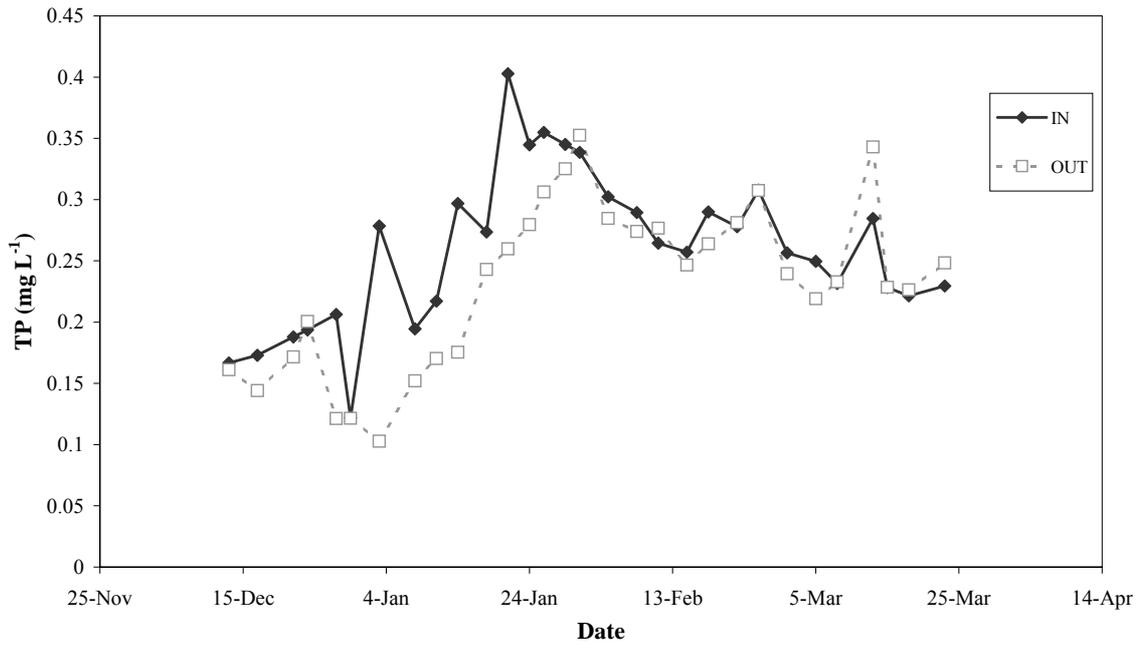
**Figure 10.** Total phosphorus concentrations in inflow and outflow of the settlement pond at Farm A.
