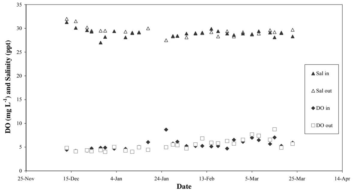
**Figure 2.** Dissolved oxygen concentrations and salinity of water flowing into and out of the settlement pond at Farm A.
