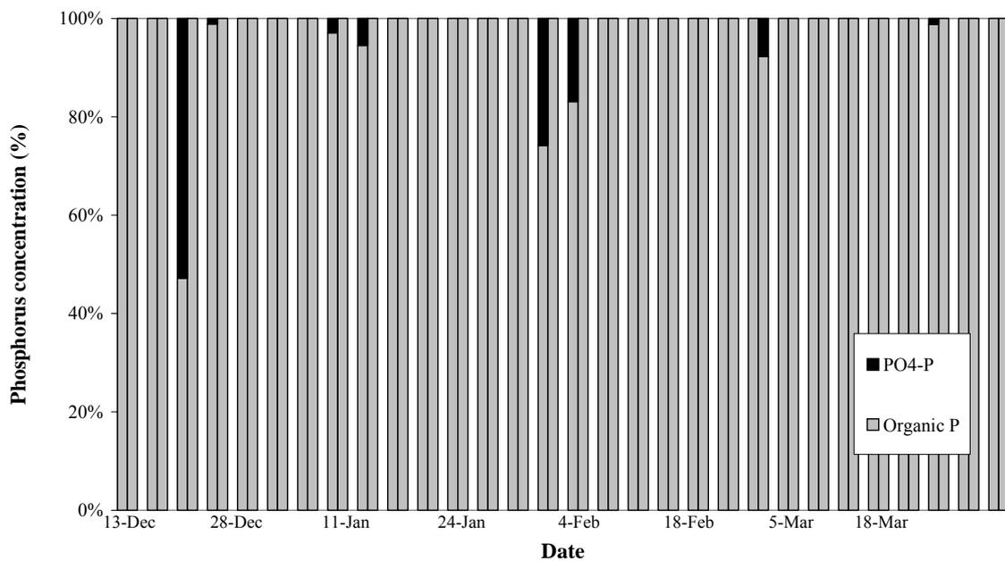
**Figure 11.** Phosphorus speciation as a percentage of the total in the inflow and outflow of the settlement pond at Farm A (Paired columns represent inflow on the left and outflow on the right).
