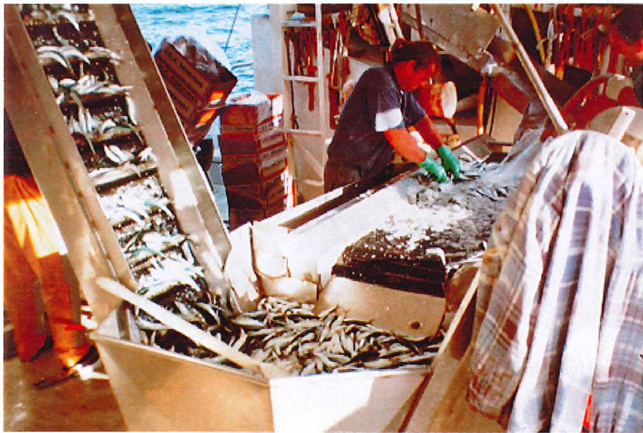
Figure 2.3. The conveyor belt leading to the "IQF" freezer.
