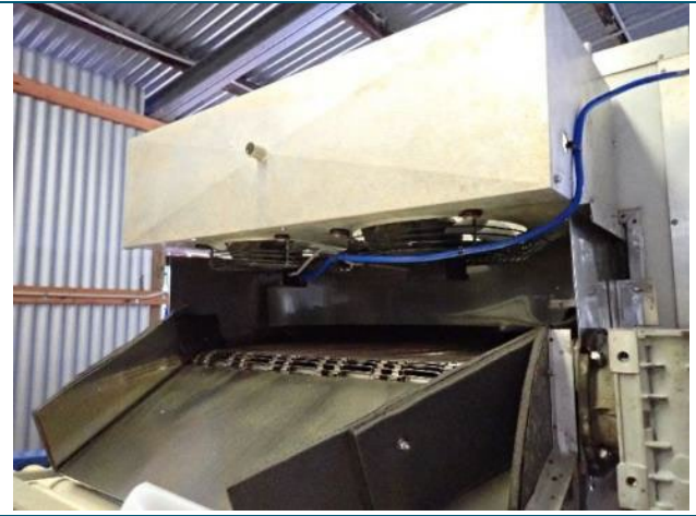
Fruit exit the hydrocooler, under an airblast to remove excess water and onto the grading conveyor.
