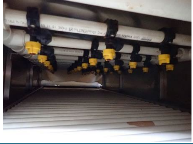
32 nozzle unit (8 rows x 4 nozzles per row)
