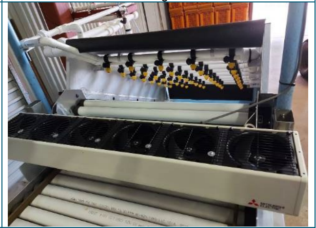
View at the top and exit point from the HPW. Fruit exit under an air blast to remove excess water before the grading conveyor.
