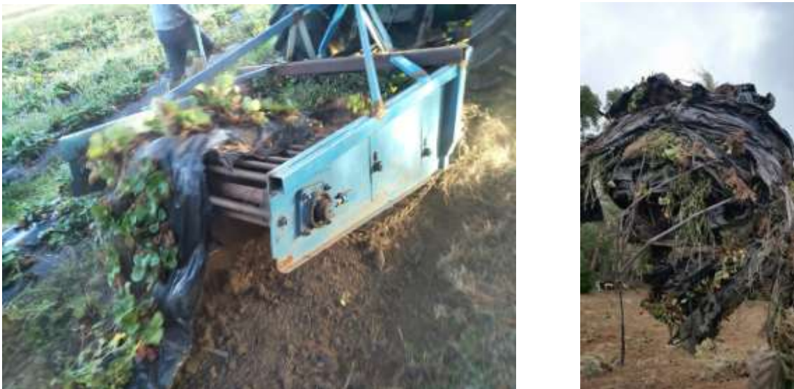
Figure 9. Machine designed by strawberry growers to remove old plants and plastic, based on the recommendations from this project.
