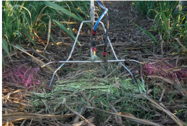
Figure 4. Final production version spraying dye in 1.8 m sugarcane rows. Yellow represents interrow glyphosate application and red row-spray application.
