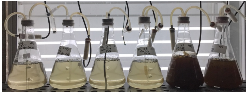
Figure 2. Heterosigma sp. culture in 2L conical flasks containing 1.6L of GSe medium.
