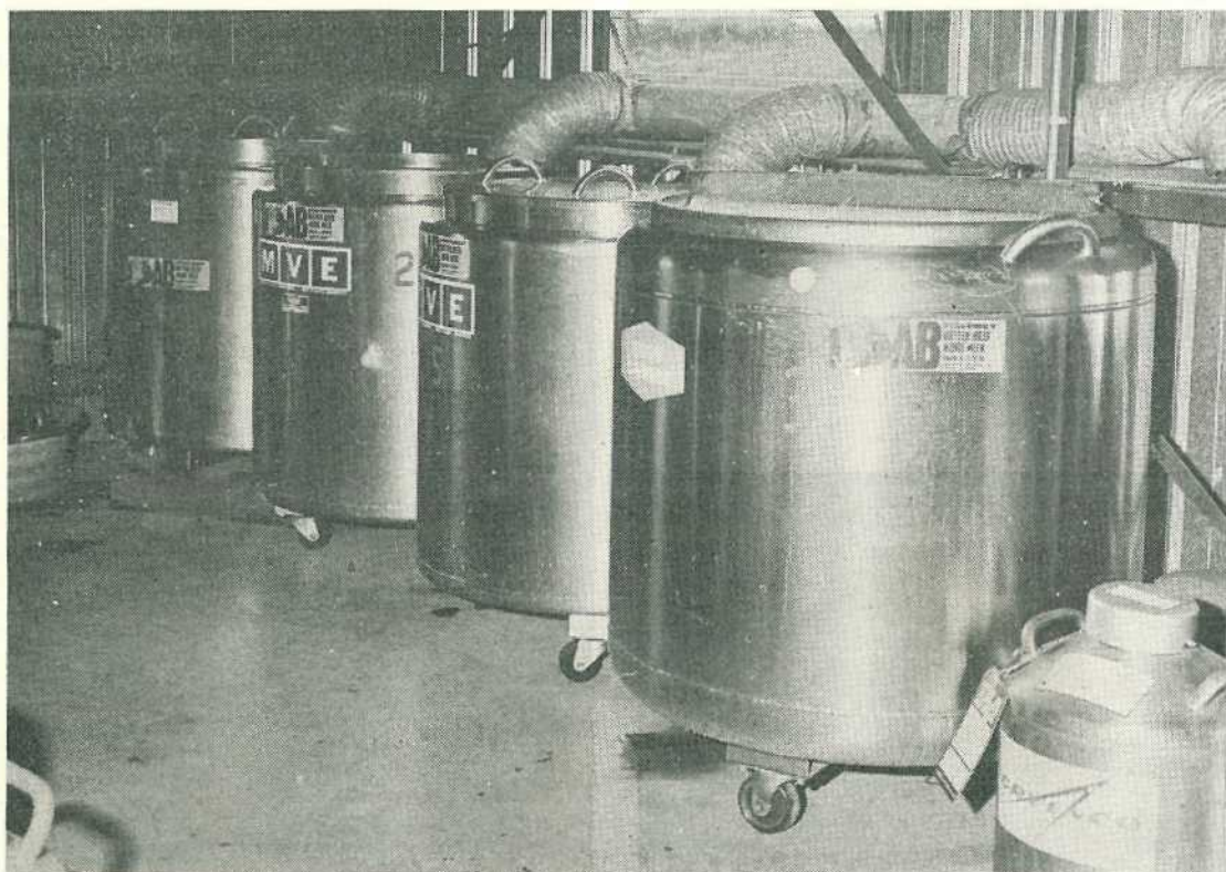
The large storage tanks each hold 250 litres of liquid nitrogen and can accommodate up to 80 000 doses of frozen semen.
