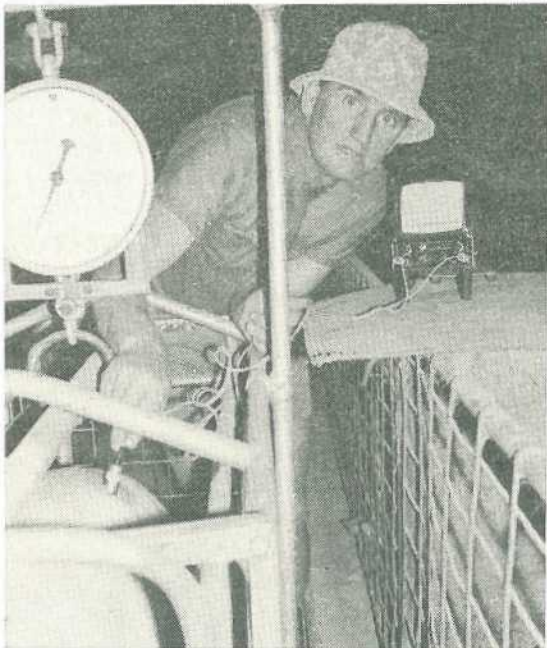
Mr. Bob Duckett shows how, with the pig restrained, the probe is held in the correct position to obtain a reading. Backfat thickness is recorded in millimetres on the face of the instrument.
