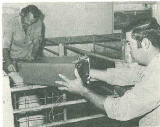
At the Rocklea Pig Test Station the electronic grader has been in use for several years. The pictures show marking of key points on the pig's back (top), placing the probe on each of these markings (middle) and reading of data from the machine (bottom).
