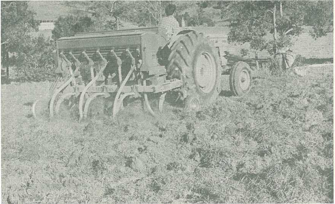
Sod-seeding ryegrass, clover and oats into a mat grass sward after rotary-hoeing.
