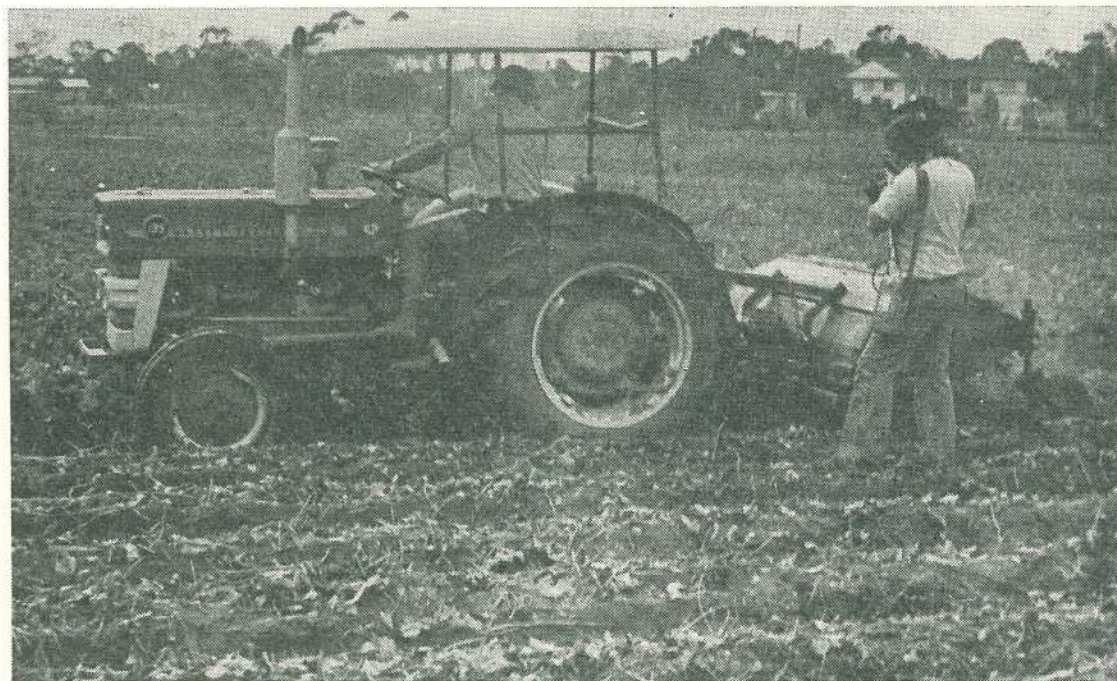
A flail type pulverizer stripping the vines off the rows preparatory to using the mechanical digger. The flails are set to fit the contours of the rows.
