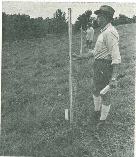
Surveying the line. The extended leg will be on the lower ground when the water columns agree.
