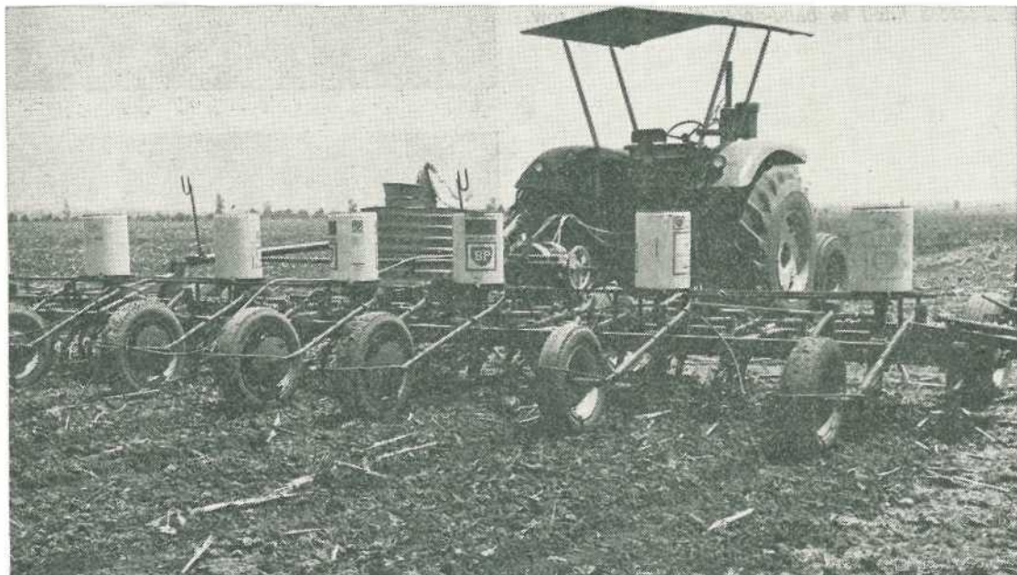
A Shearer wideline cultivator modified for sorghum planting on the Hill Brothers' property at Yelarbon. Combine seed distributors have been attached to oil drums to produce row planting units.
