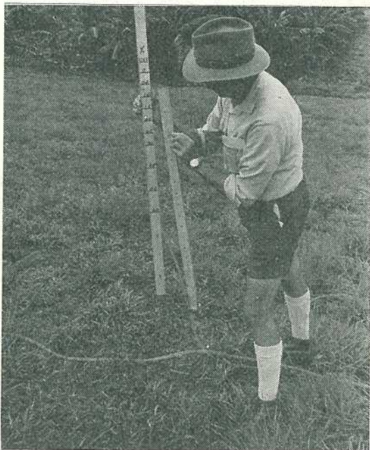
Adjusting the extension leg to the desired gradient. The percentage gradient is marked on the staff above the extension leg.
