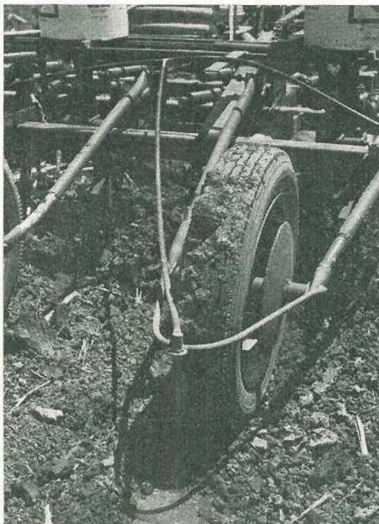
These home-made presswheels have herbicide applicators fitted to band-spray the sorghum row.
