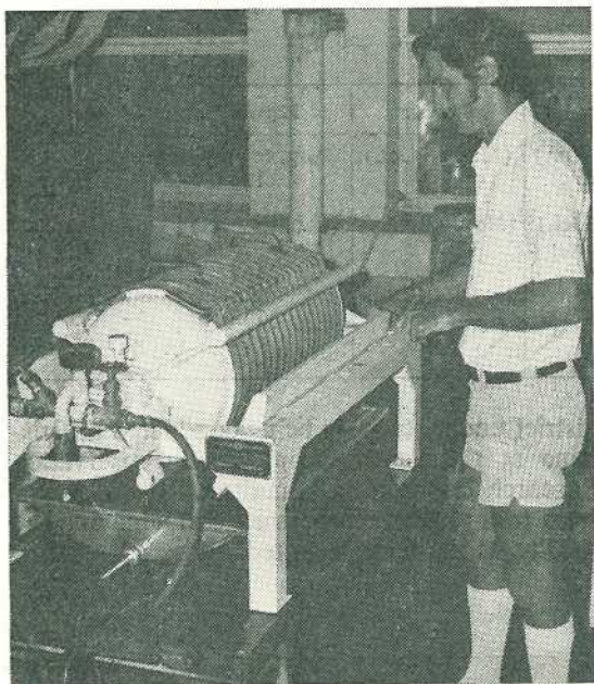
ABOVE: Dennis McEvoy separating skins from wine in a pilot scale Willmes press at the Department's Hamilton laboratories.
