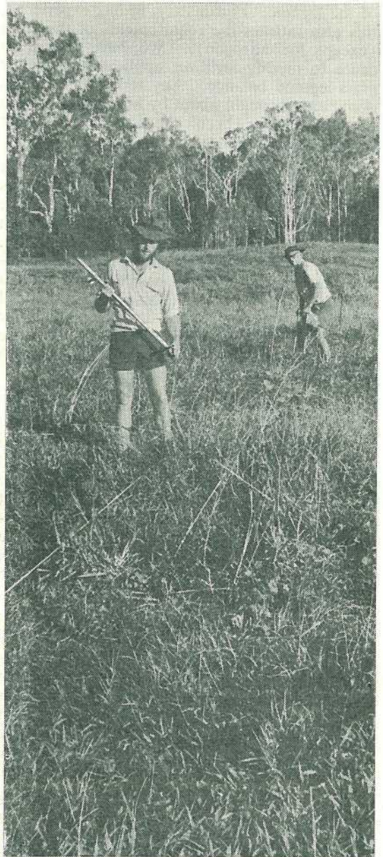
Soil sampling prior to fertilizer application with a 'Jarret' auger along a transect marked with a string.
