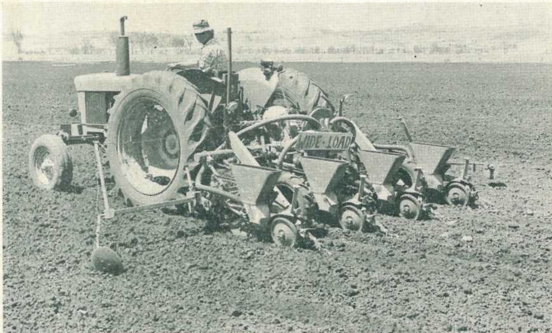
A vacuum-operated precision planter produces uniform plant stands.
