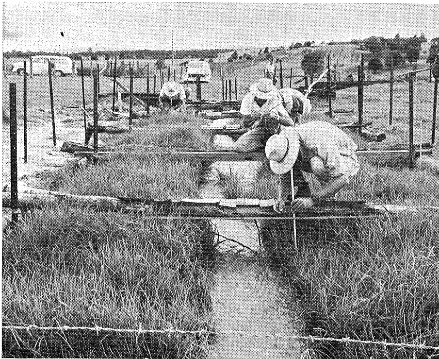
Fig. 4.—Measurement of water surface being made at four stations during a test flow (Test 1).
