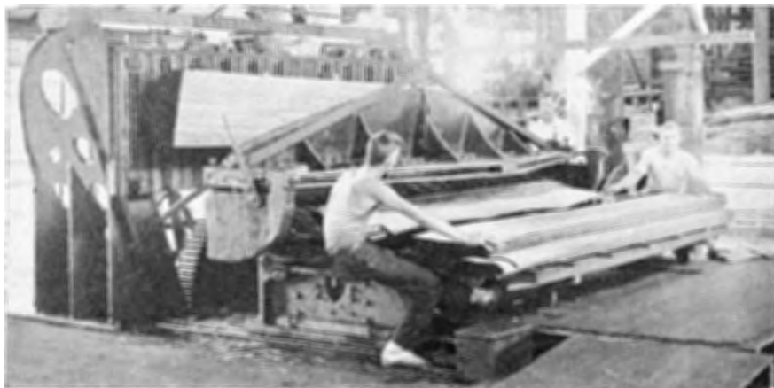
Veneer-slicer in Operation, Cairns, North Queensland.
