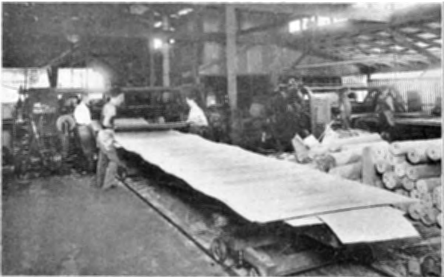
Peeling Hoop Pine Logs on Rotary Lathe.
