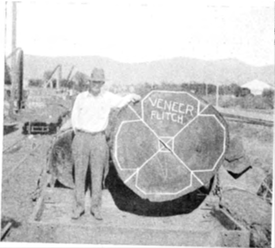
Queensland Walnut Log Marked for Sawing into Flitches for Quarter-slicing.
