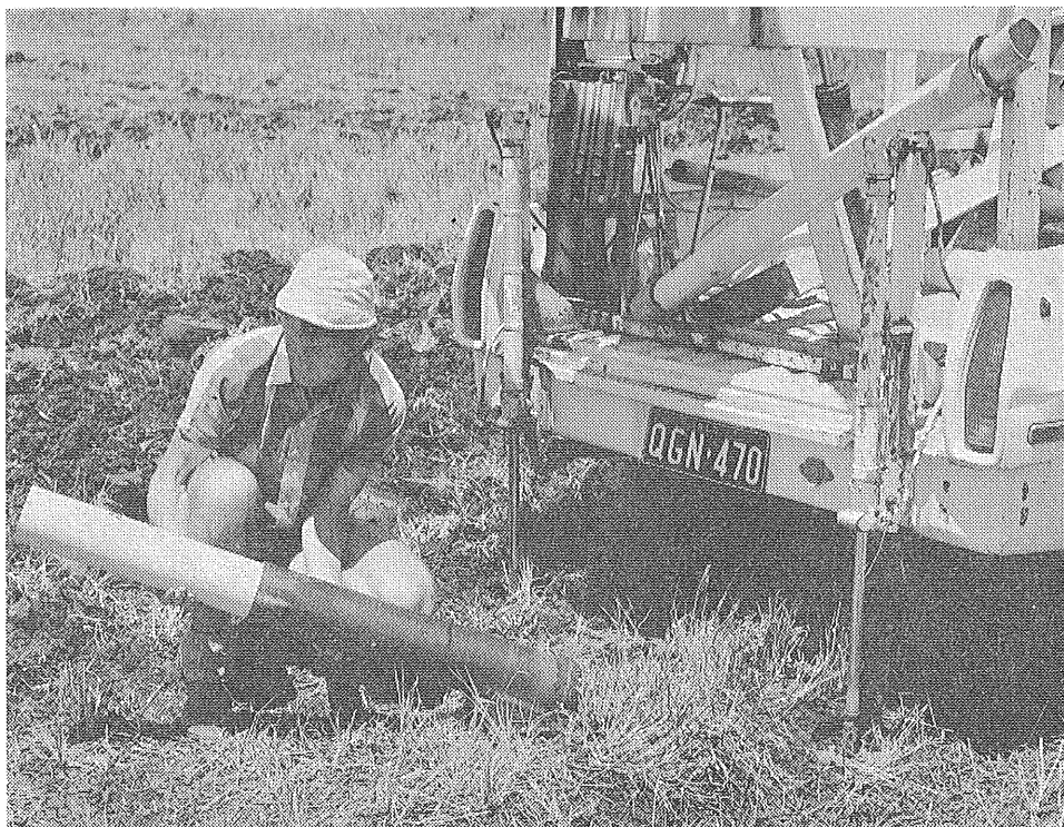
Figure 3.—Removal of PVC liner containing core from the sampling tool.
