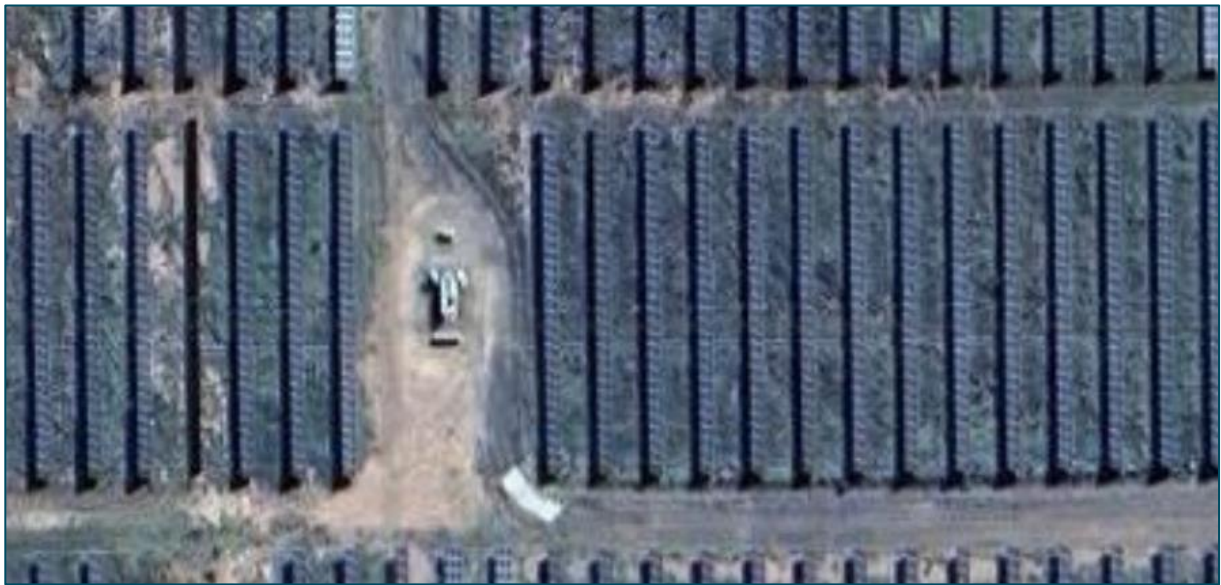
Figure 3 Closer view of panel arrangement and spacing at Lilyvale Solar Farm in central Queensland, near Tieri (Google earth imagery; downloaded 06/02/2024)
