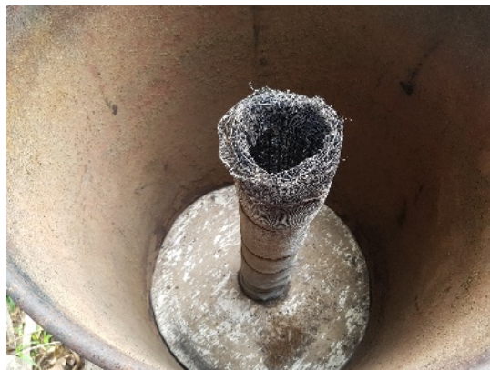
Plate 1b. Plywood base and vented flue to distribute steam
