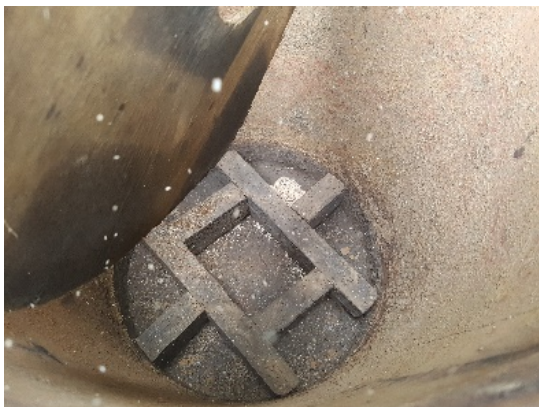
Plate 1a. Water compartment at base of 200 L drum with wooden spacers for the plywood base.
