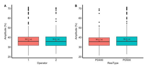
**Figure 5.** Variation in Resi amplitudes detected for seven IML Resi tools. (**A**) Resi amplitude between two operators. (**B**) Resi amplitudes detected for the two types of Resi tools (PD400 and PD500) used in the study. Means with a common letter are not significantly different.
