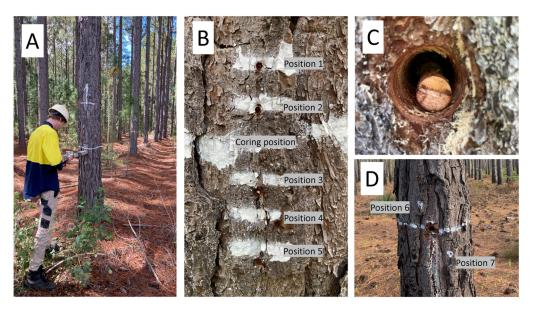
**Figure 1.** (**A**) Sampling trees at DBH 1.3 m with Resi in the plot. (**B**) Allocated sampling and coring positions on the tree with visible Resi holes. (**C**) Drilled 12 mm diameter and 50 mm length core in the outerwood in the tree. (**D**) Additional Resi sampling positions added after the core has been taken.
