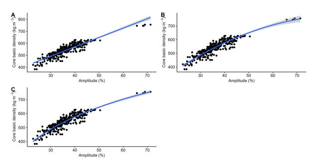
**Figure 4.** Modeled test data from a randomized 80/20 split of the data from the seven Resi tools: (**A**) linear model; (**B**) power model; (**C**) natural log model.
