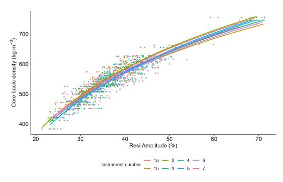
**Figure 6.** Resi amplitudes detected for seven IML Resi tools used in the study. Instrument 1a and 1b are the same Resi tool used as new and post-servicing by IML.
