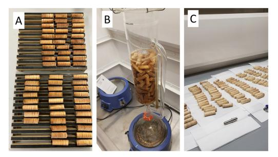
**Figure 2.** (**A**) Green 50 mm length and 12 mm diameter cores before extraction. (**B**) Removing extractives using a soxhlet extraction apparatus set up in a fume hood. (**C**) Cores after extractives have been removed.
