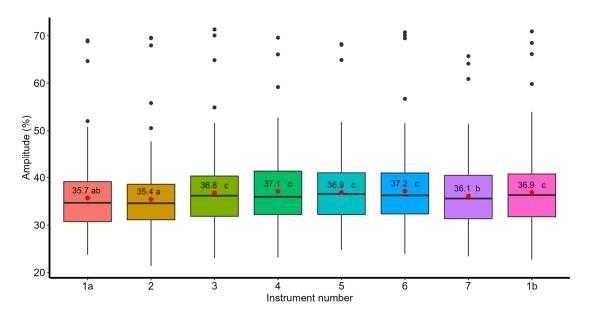
**Figure 7.** The mean values of Resi amplitudes (50 mm from Resi entry) for seven instruments across the sites. Instruments 1a, 2, 3, 4, and 5 were tested in April, instrument 6 in June, and instruments 1b (post service of instrument 1) and 7 in November, with sampling positions further from the core location. Means with a common letter are not significantly different.
