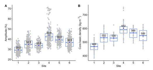
**Figure 3.** (**A**) Box plot of Resi outerwood amplitude for each site using all seven IML Resi tools. (**B**) Corresponding 50 mm outerwood core-extracted basic density for each site. Mean values are represented by blue dots.
