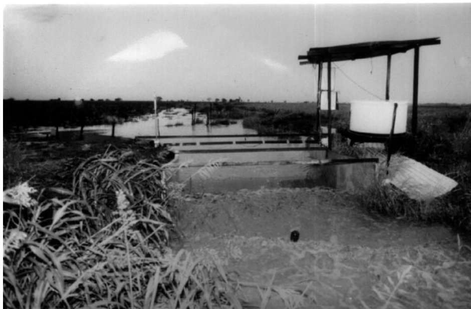
Fig. 3. Parshall flume at outlet of contour bank. Sediment sampling arm is seen in flow. Sediment dispenser is positioned on the right of the flume (white container).
