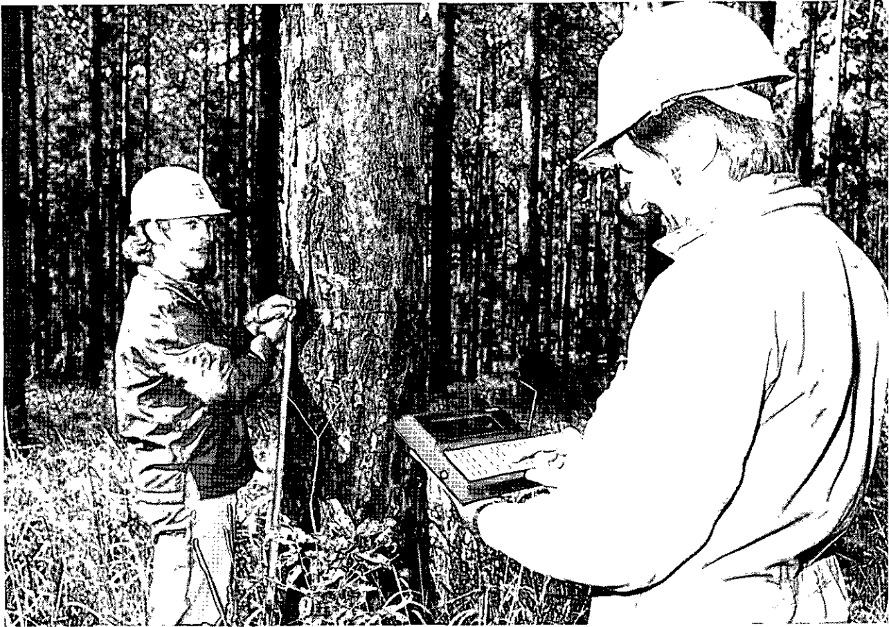
Forest overseer Noel Faulkner (right) and assistant Brian Neylon record slash pine measurements on a hand held data capture device as part of an inventory sampling procedure to gather base standing volume figures and to project yields.
