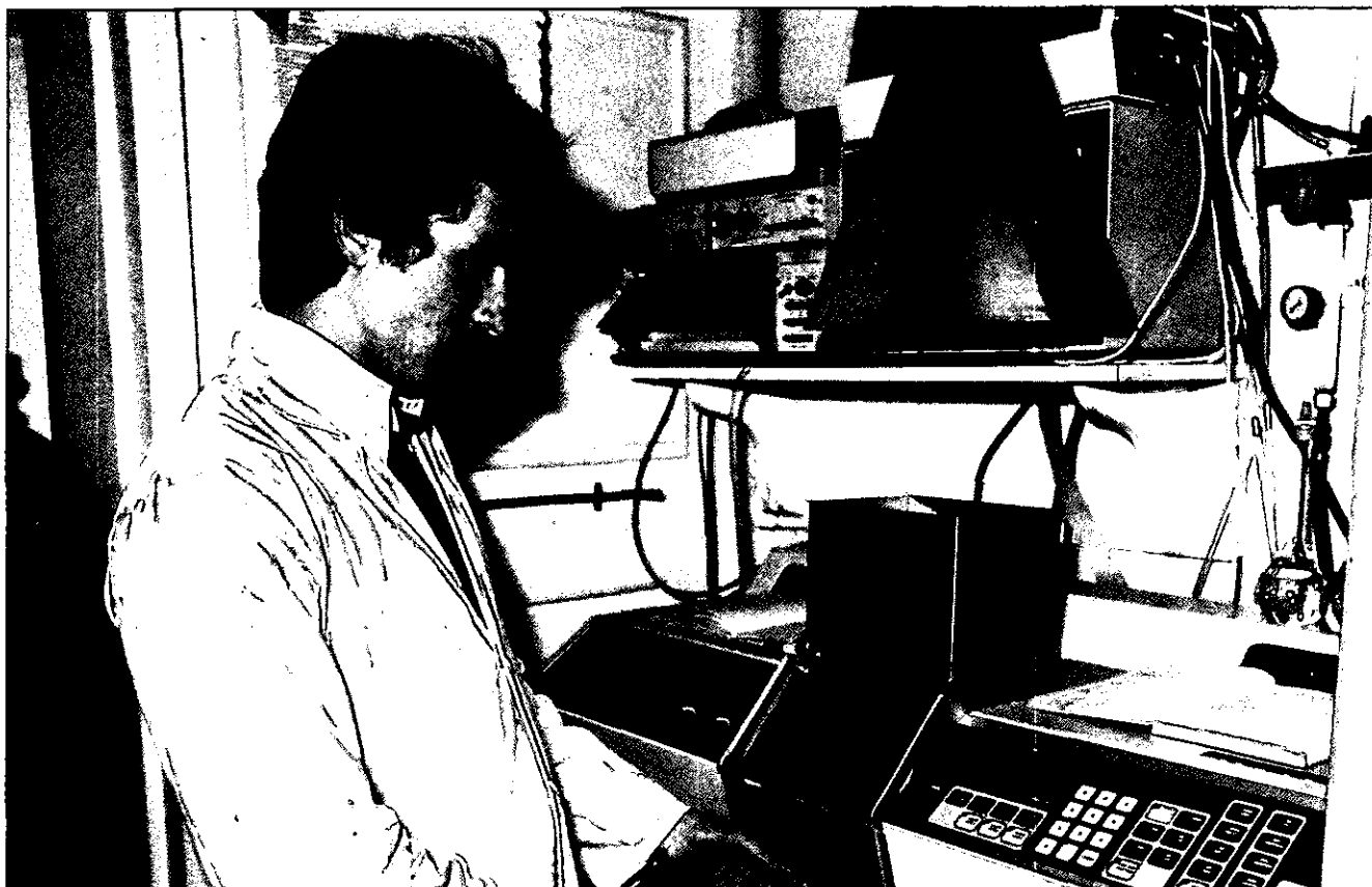
Laboratory Technician Robin Davis testing samples in an atomic absorption spectrophotometer.
