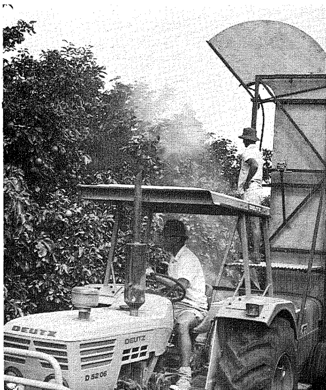
A 'Towermister' air blast sprayer allows good all-over coverage of citrus trees.
