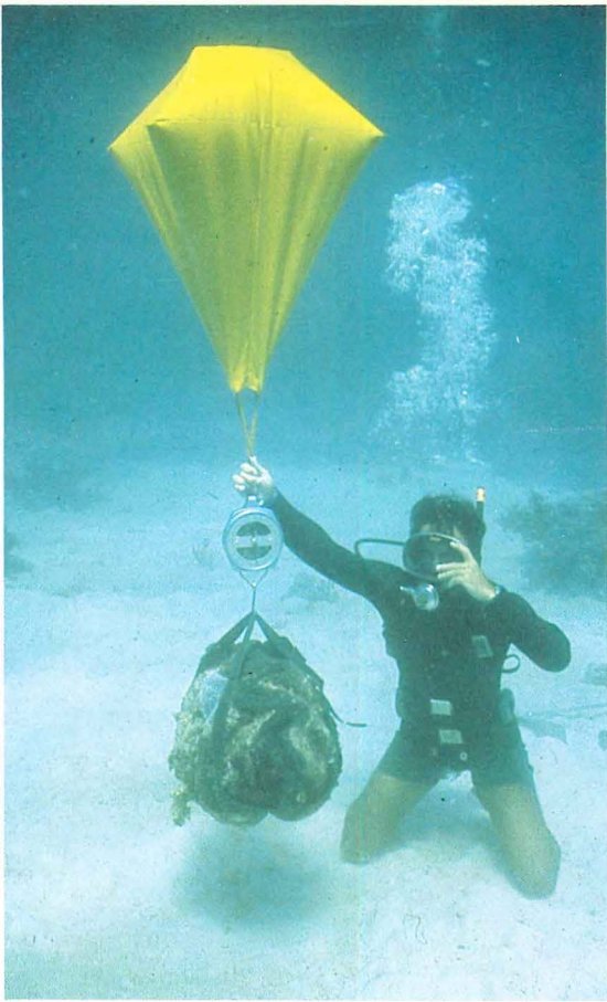
A Fisheries Research Branch diver weighs a giant clam under water, using a spring balance suspended from an air bag.
