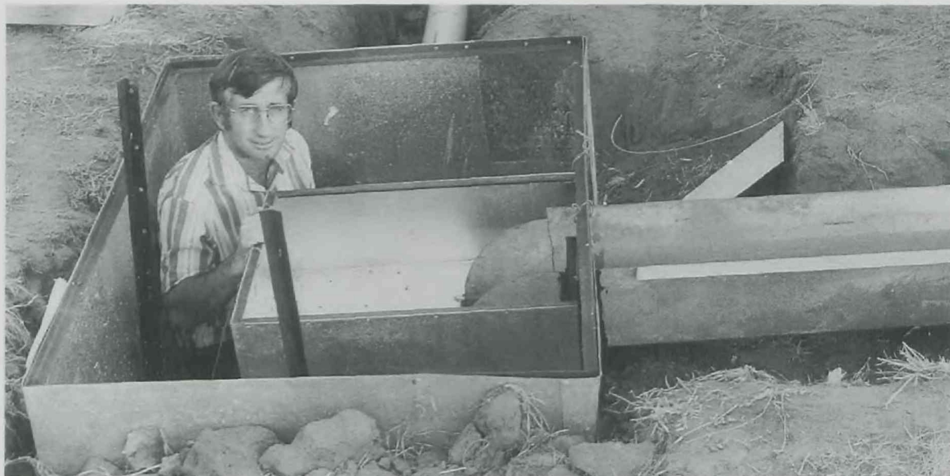
A DPI experimentalist at Ayr tests the operation of the 'tip bucket' on a rainfall runoff measuring system. Twenty of these are installed in the Mingela-Charters Towers area.
