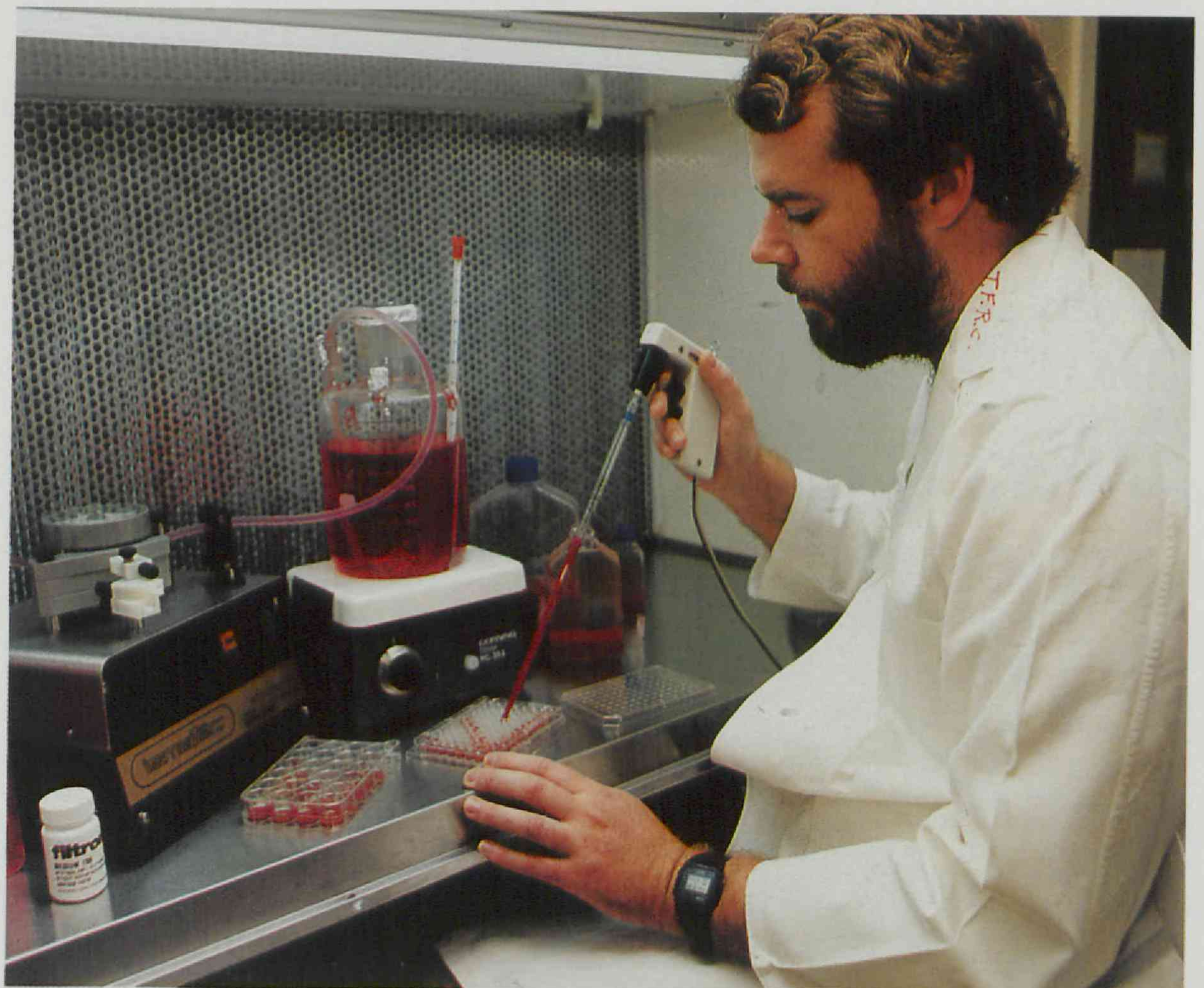
DPI scientists culture Babesia parasites as part of a new technique, developed in the DPI's Animal Research Institute laboratories, to produce cattle tick fever vaccine.
