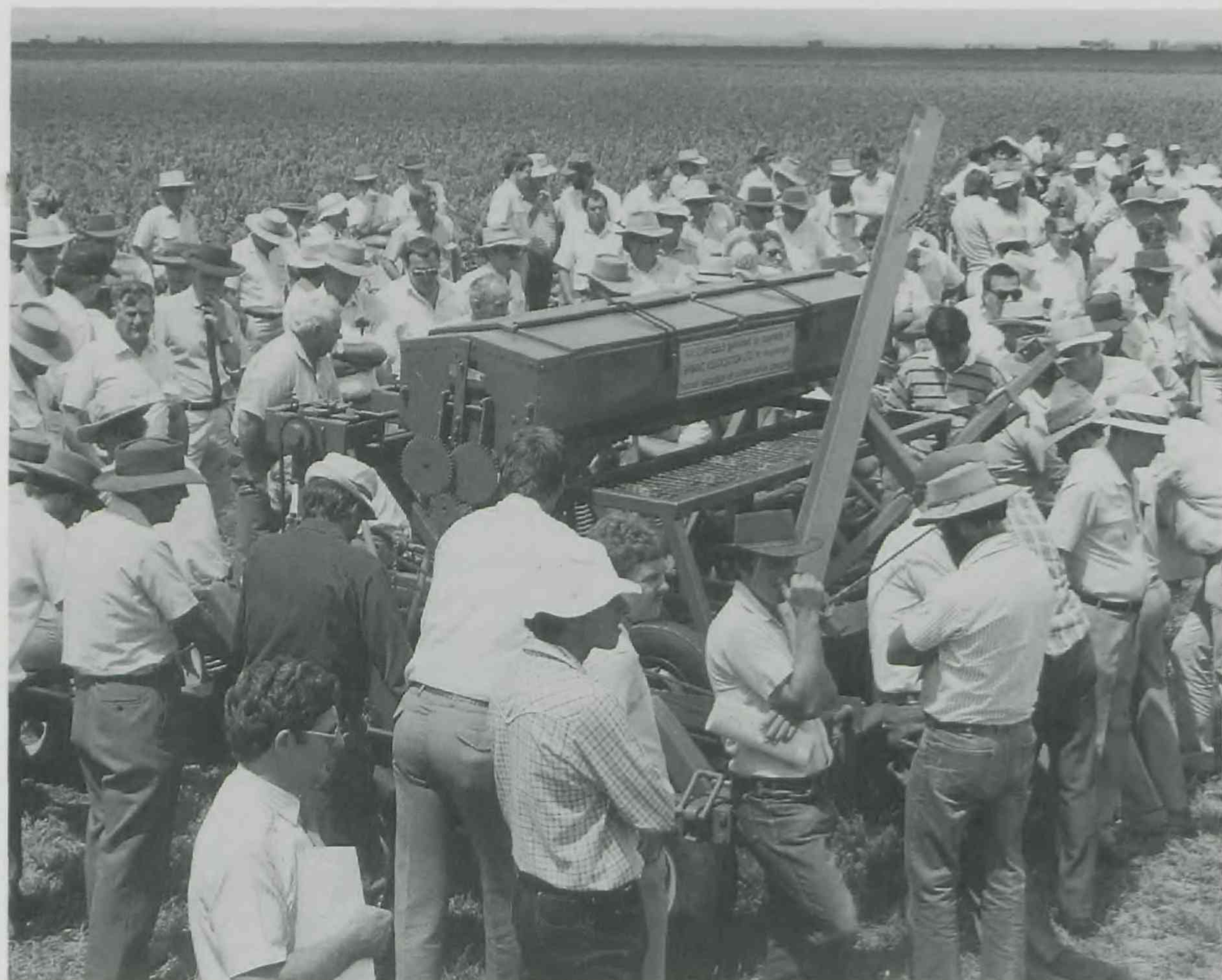
Growers inspect a reduced tillage planter developed and built by DPI staff. It was successfully used to plant oats on the western Darling Downs in both reduced and zero-tilled situations.
