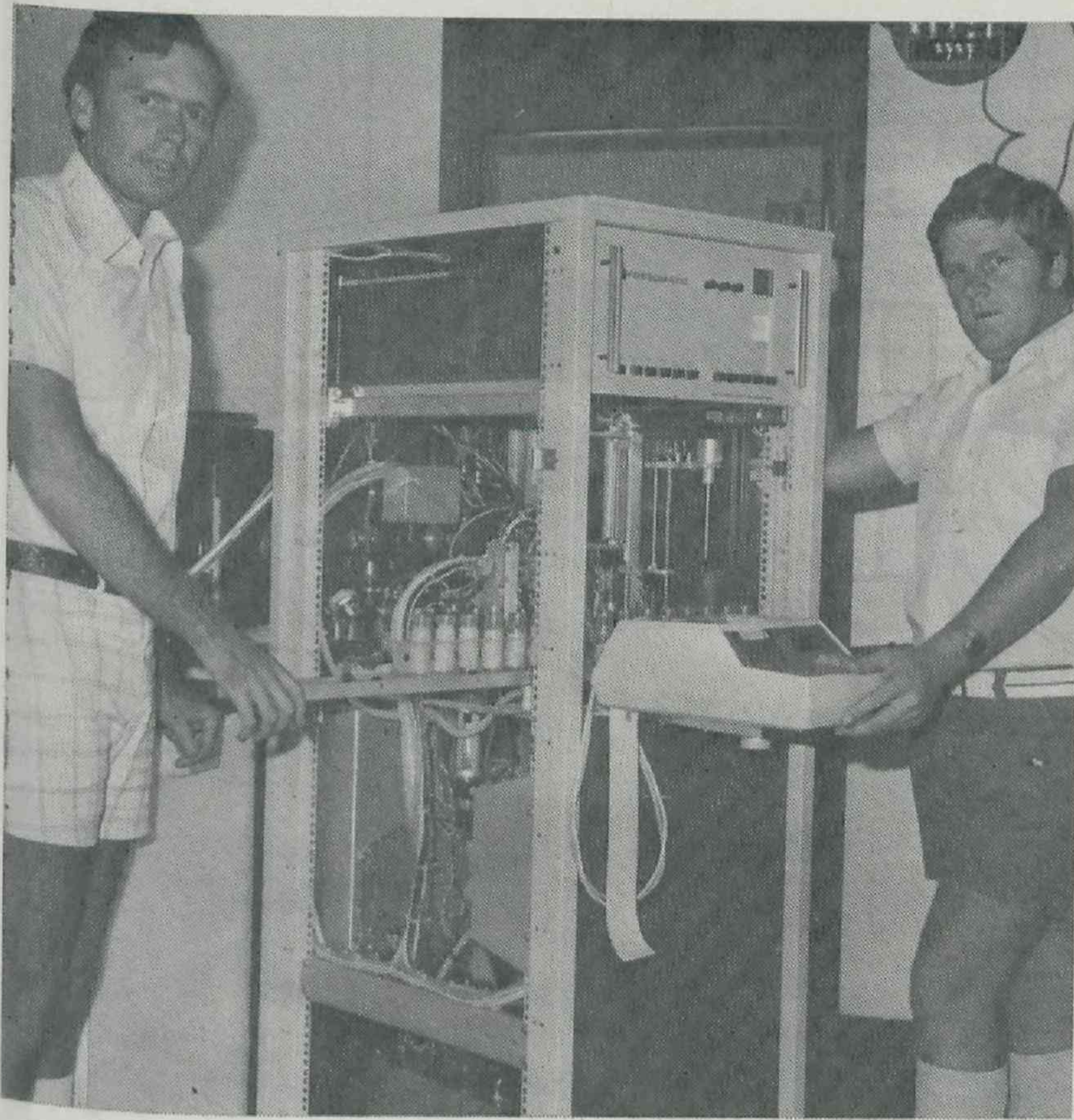
The Fossomatic somatic cell counting unit used in examining herd milks in the mastitis detection and control program.
