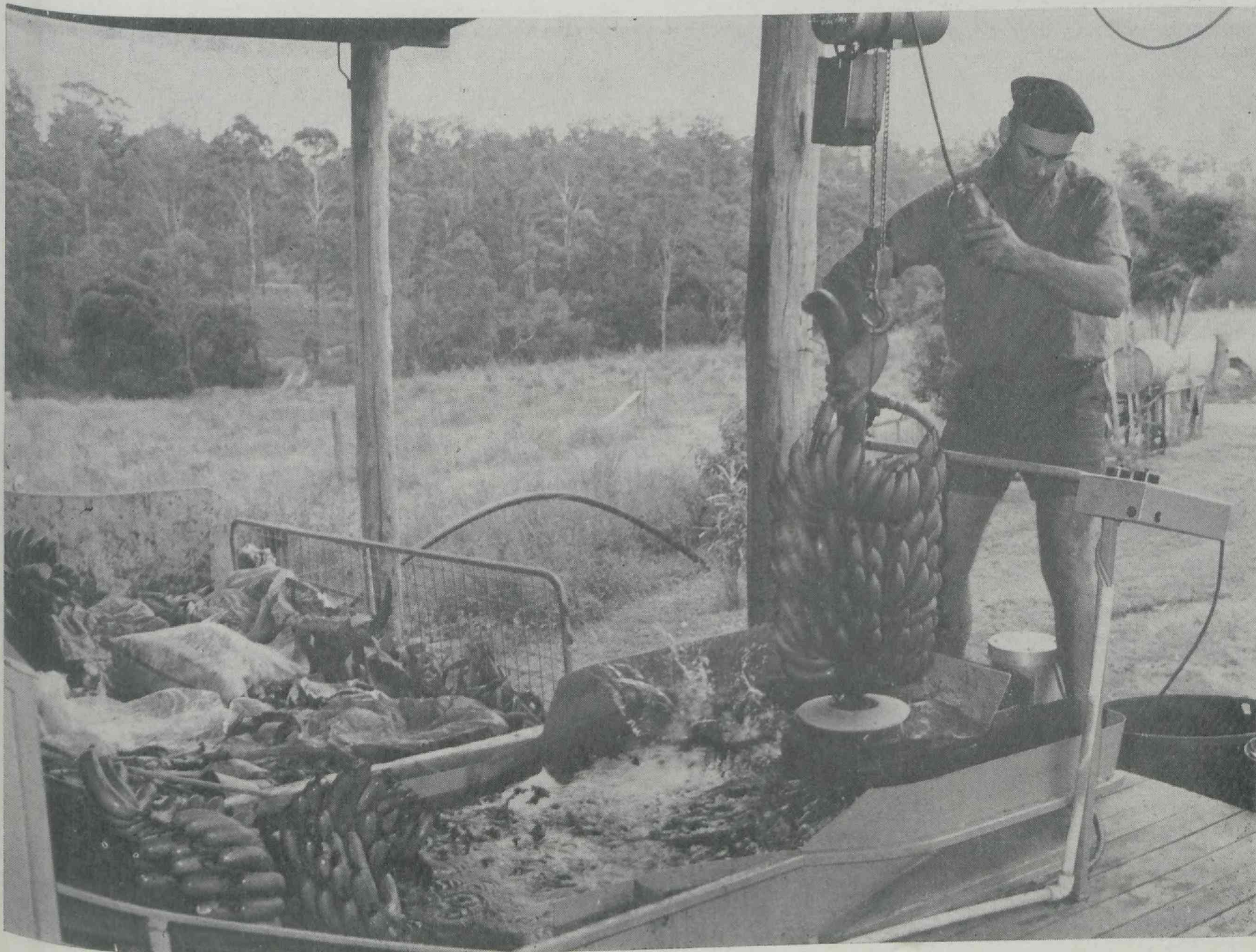
Banana grower Mr K. Lindsay, of Caboolture, demonstrates a banana dehanding machine which he designed and built.
