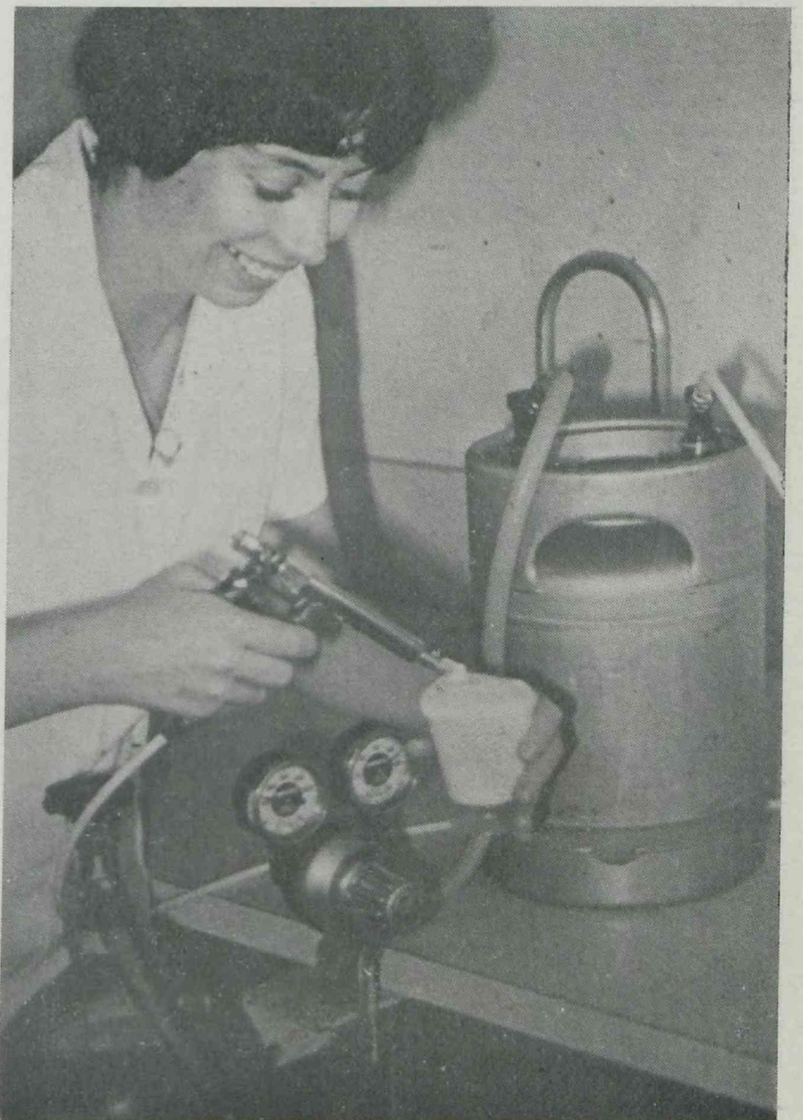
A 'cream whipping' unit designed to facilitate the addition of cream to food portions.
