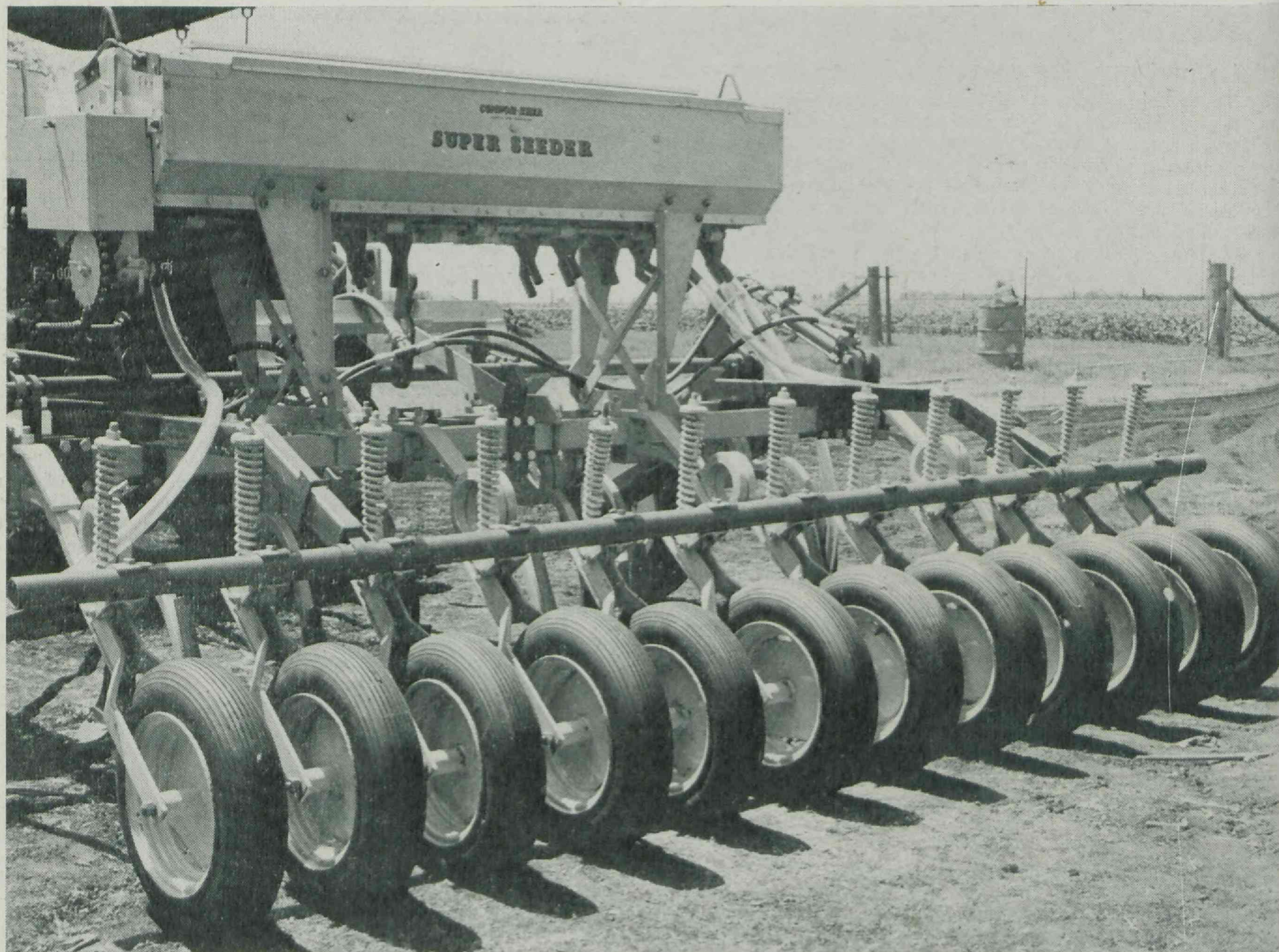
Press-wheel seeders are a major development in crop and pasture establishment.
