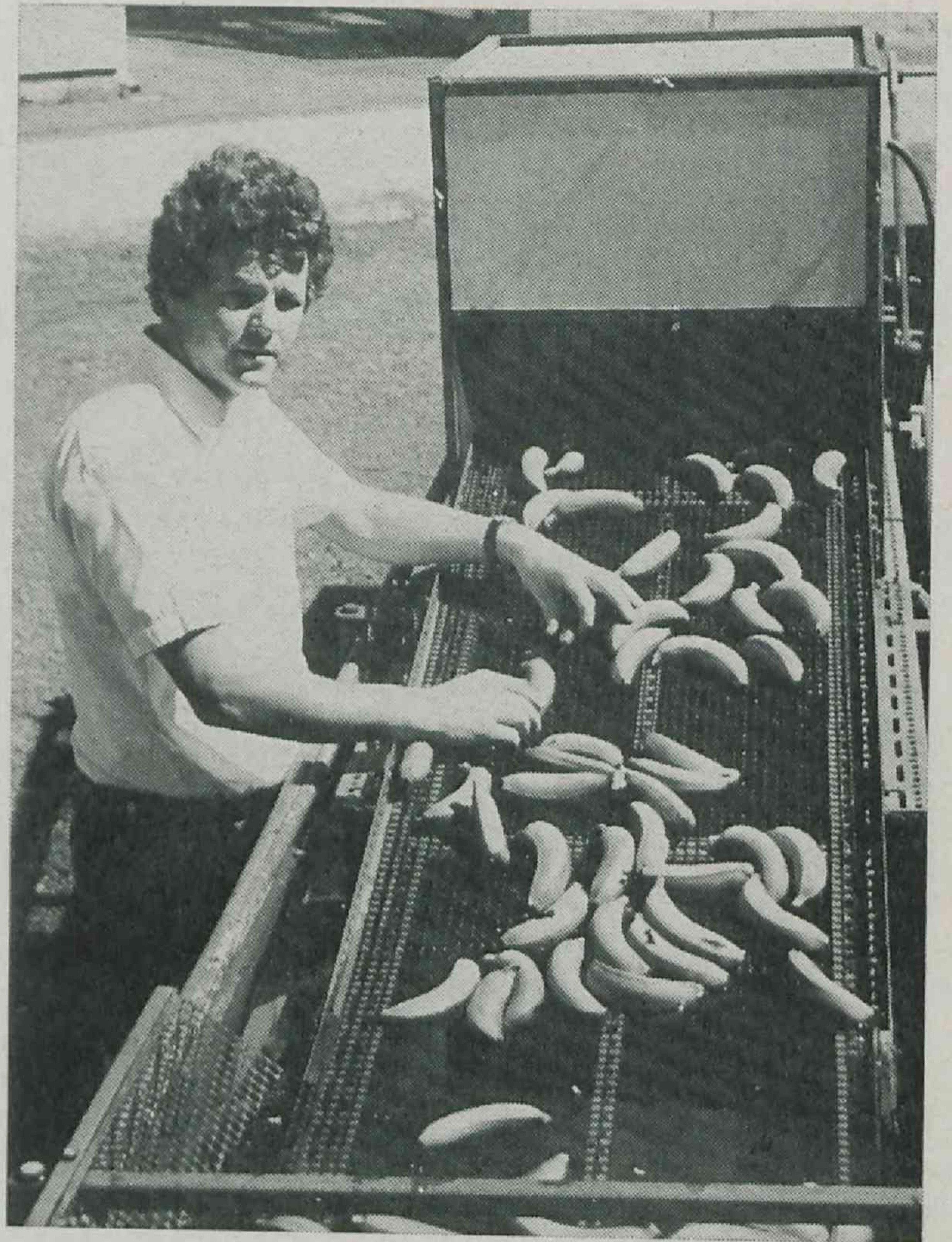
Bananas are inspected as they move along the conveyor belt of a demonstration tight-fill packaging line.
