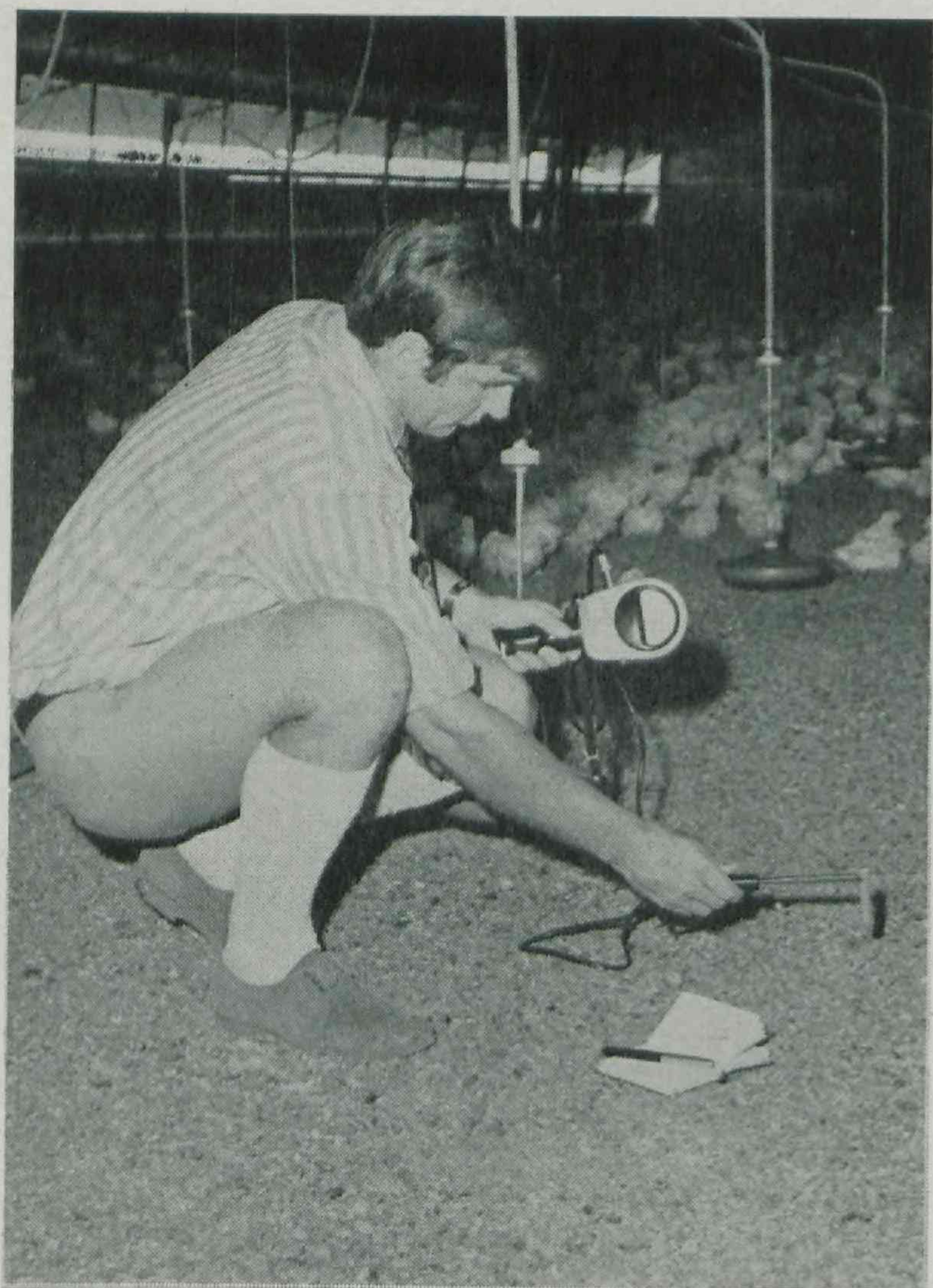
A poultry officer uses a hot wire anemometer to check air movement at floor level in a broiler shed.
