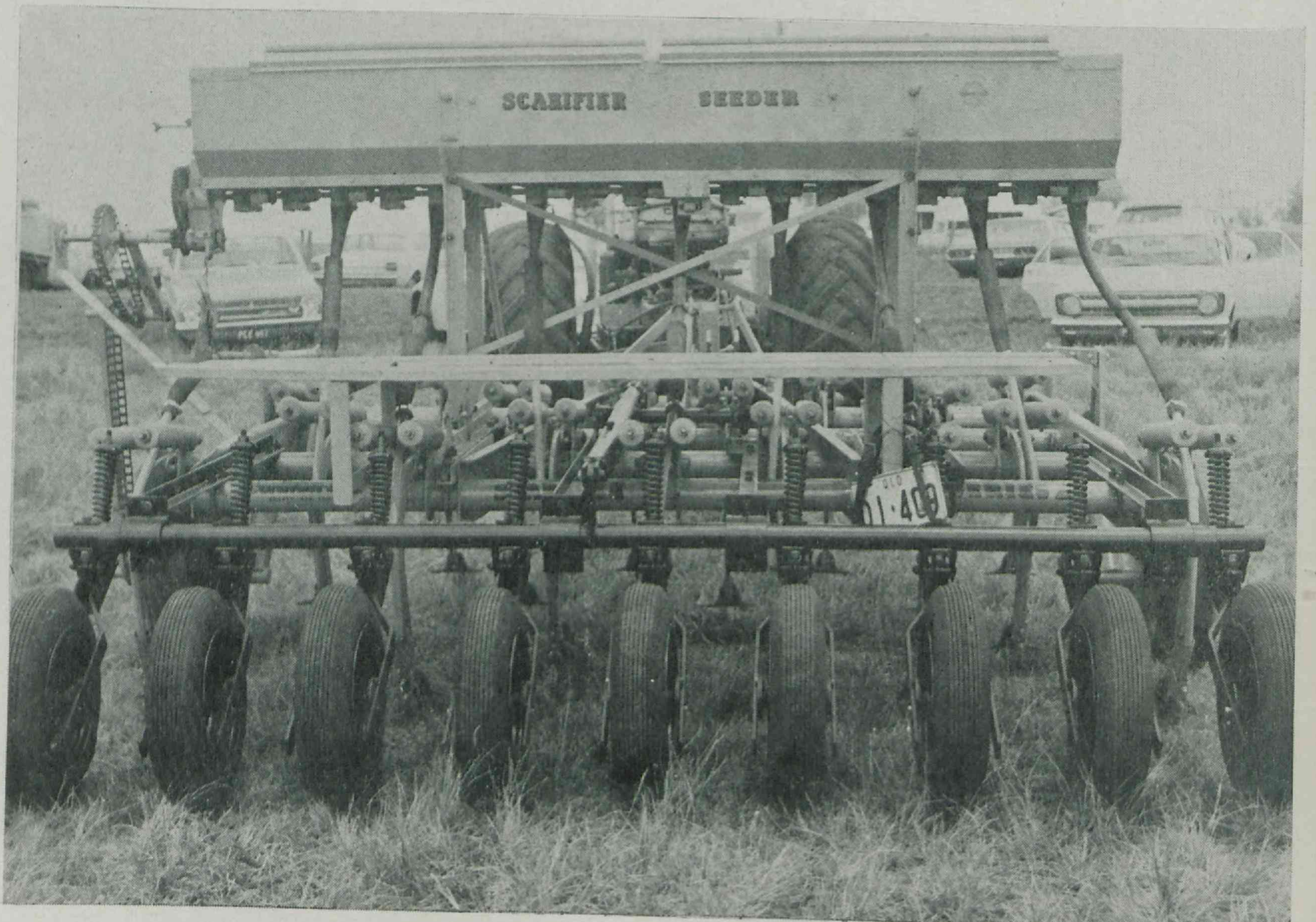
A machine adapted to plant grain through stubble and into the subsurface moisture. This technique is important in soil conservation and to give more flexibility to planting some time after rain.
