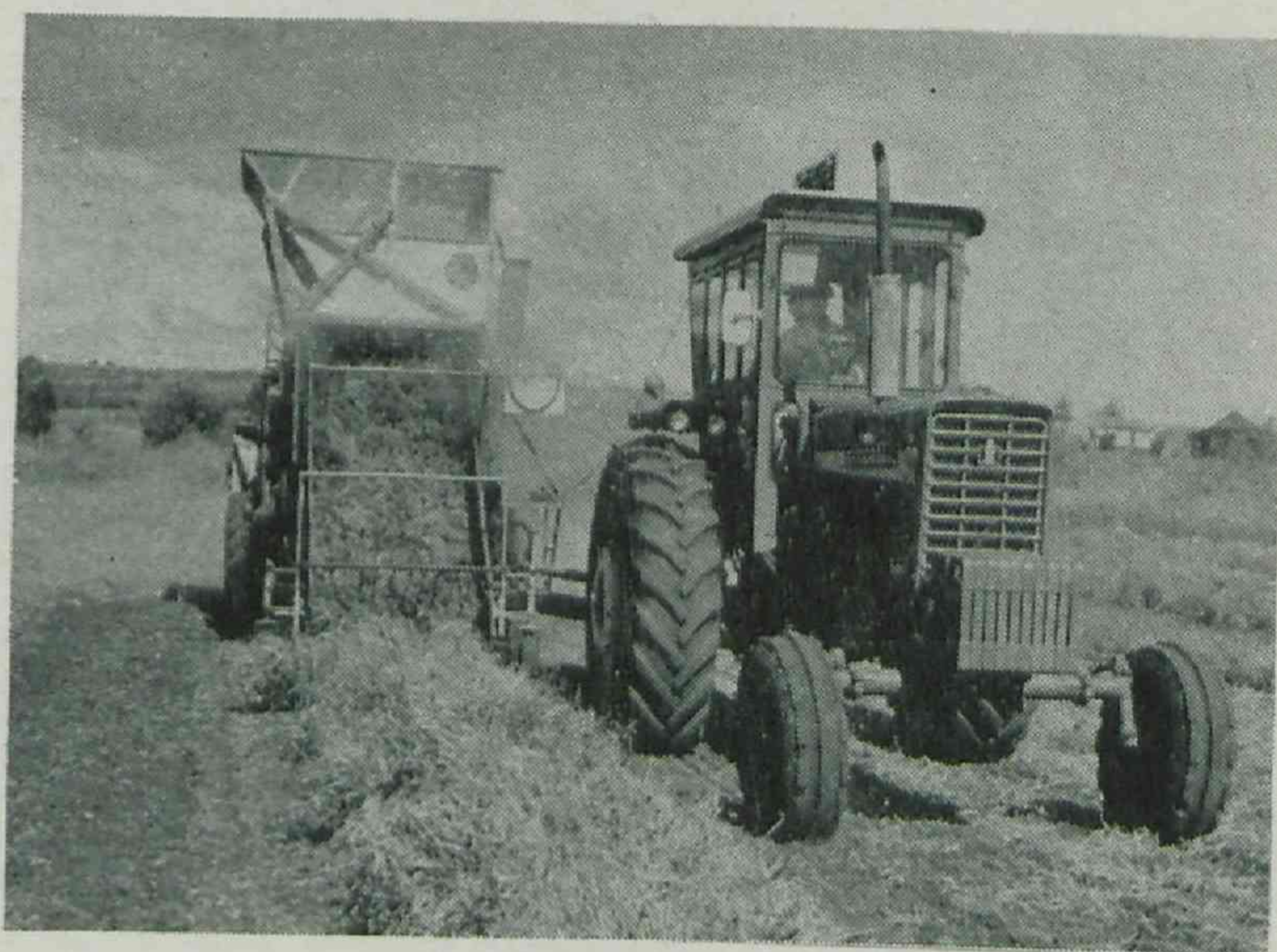
A peanut thresher modified to handle navy beans.
