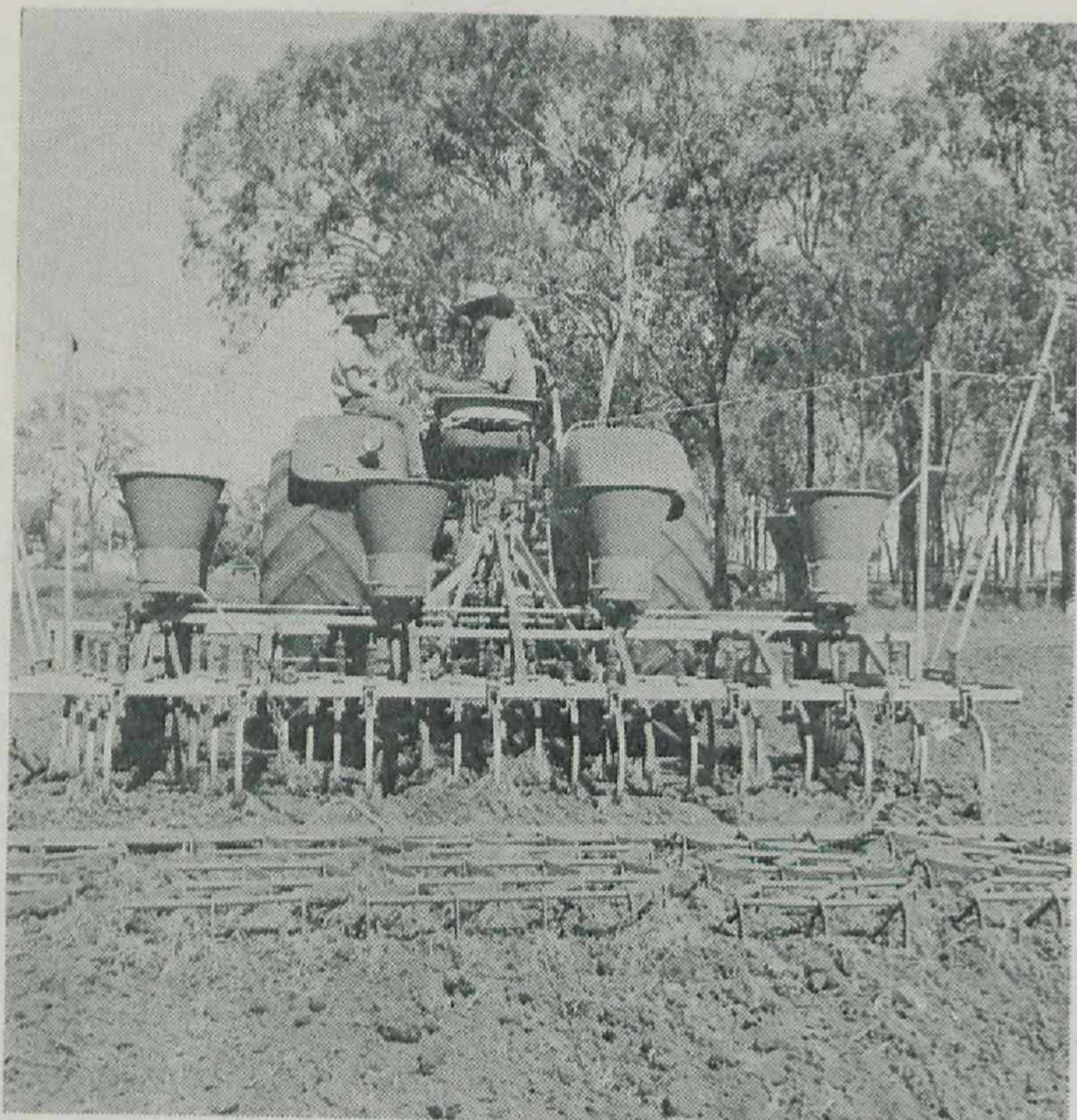
Four-row planter and fertilizer-cultivator combination used for planting navy beans and other row crops, and also for inter-row cultivation.
