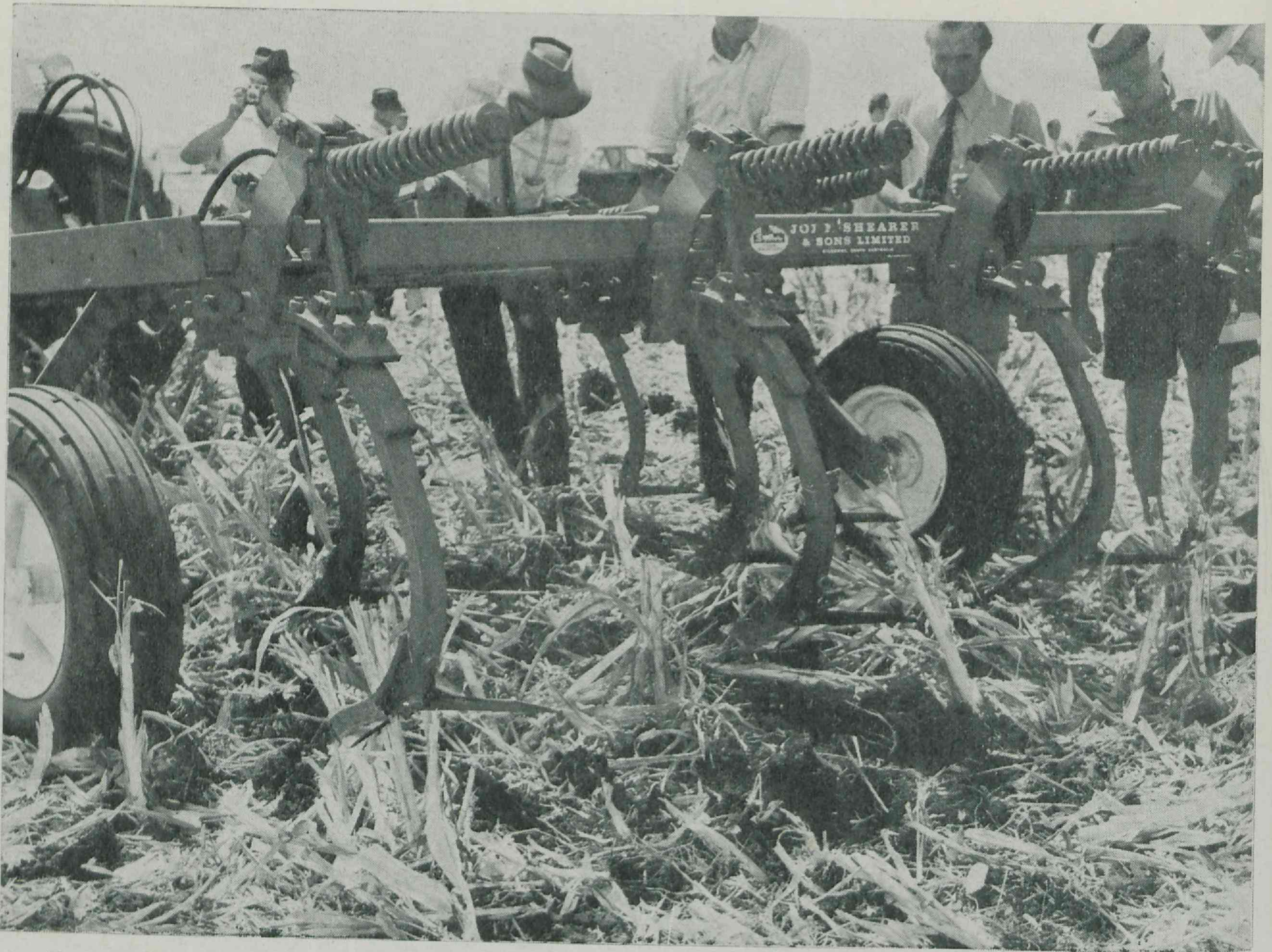
Farmers show interest in the design of a new trash chisel plough at a recent Stubble Mulch Field Day. This machine has about 75 cm under-frame clearance.
