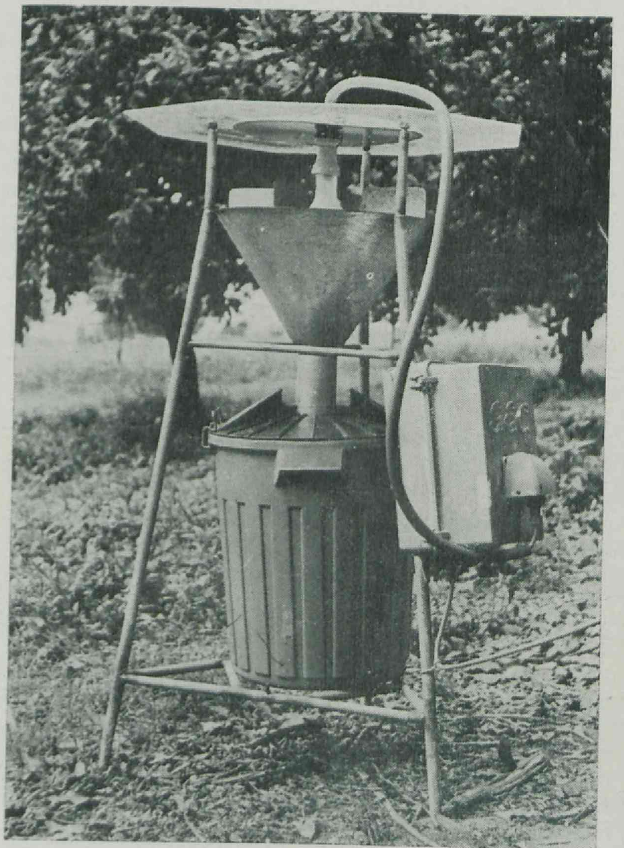
Ultraviolet light trap for the study of moth populations of macadamia pests.
