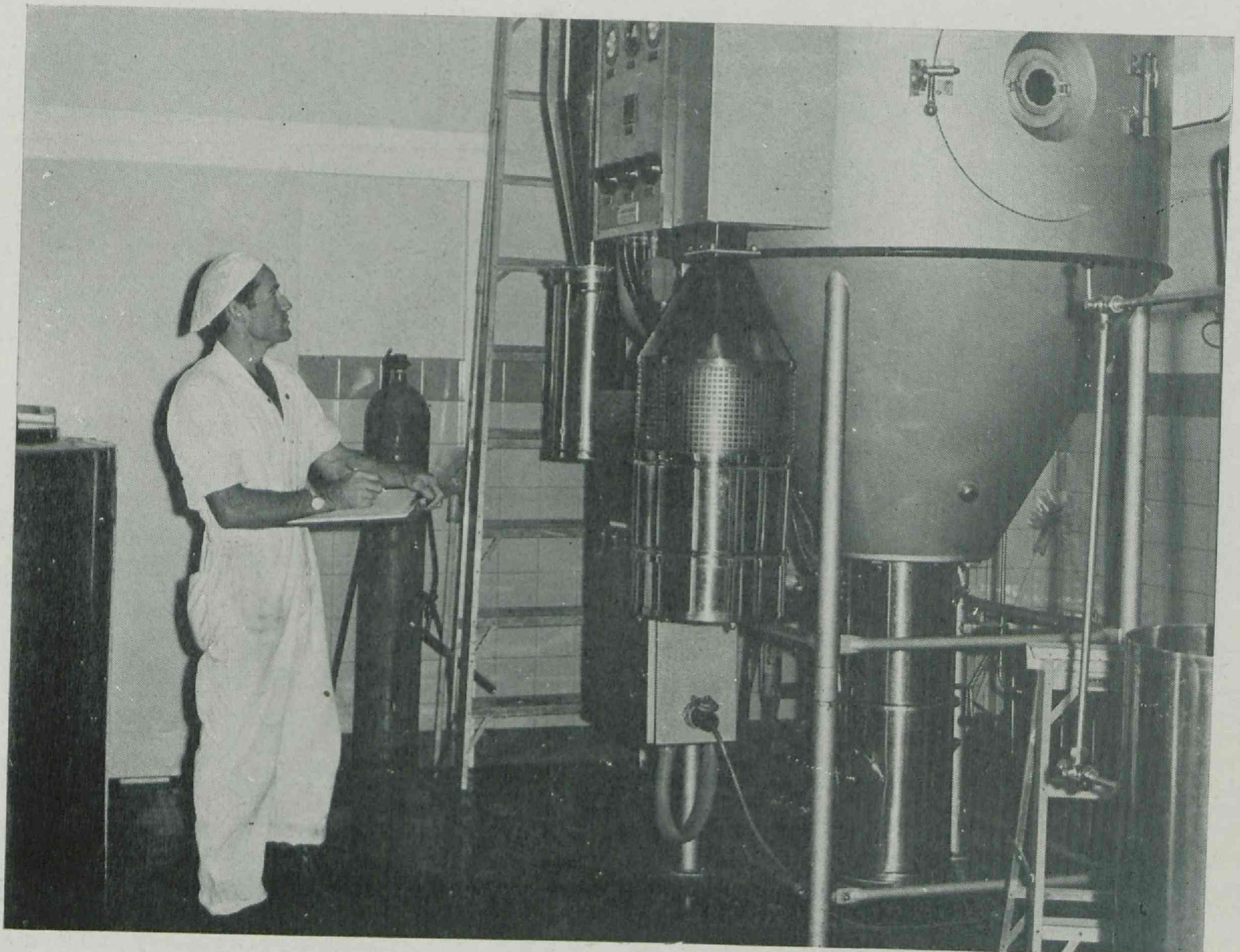
A spray drier in use in the Department's Dairy Pilot Plant at Hamilton.
