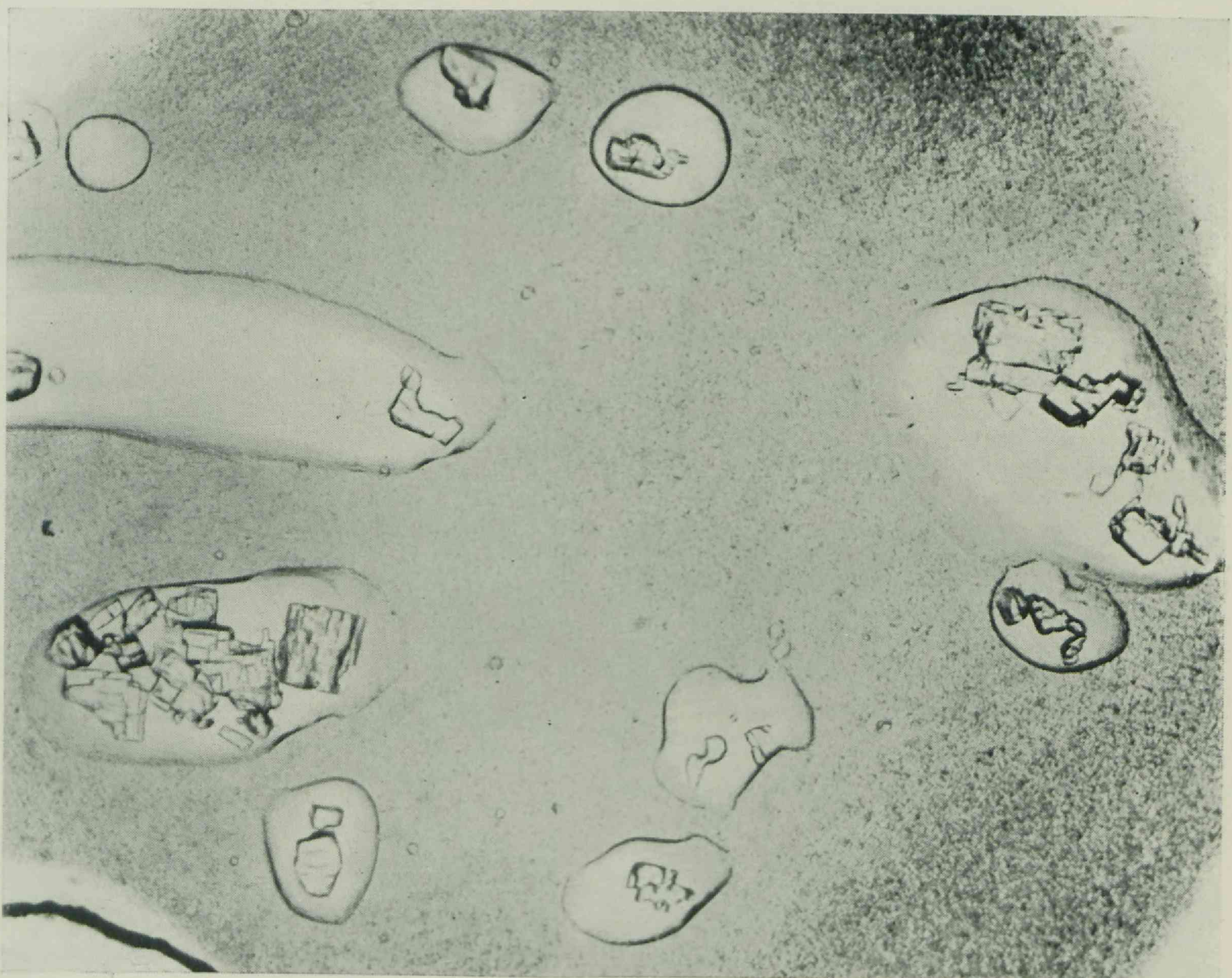
Plate 11.—The microscope reveals the cause of mottling in butter. Water migrates towards undissolved salt crystals, resulting in the formation of very large droplets. These do not reflect light to the same extent as do the normal small droplets and the butter appears mottled.
